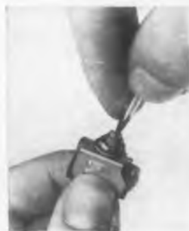
This subminiature switch assembly is operated by 90° turn of a screwdriver
