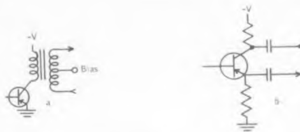
Fig. 1. Conventional driver stages for getting phase reversal using transistors.
