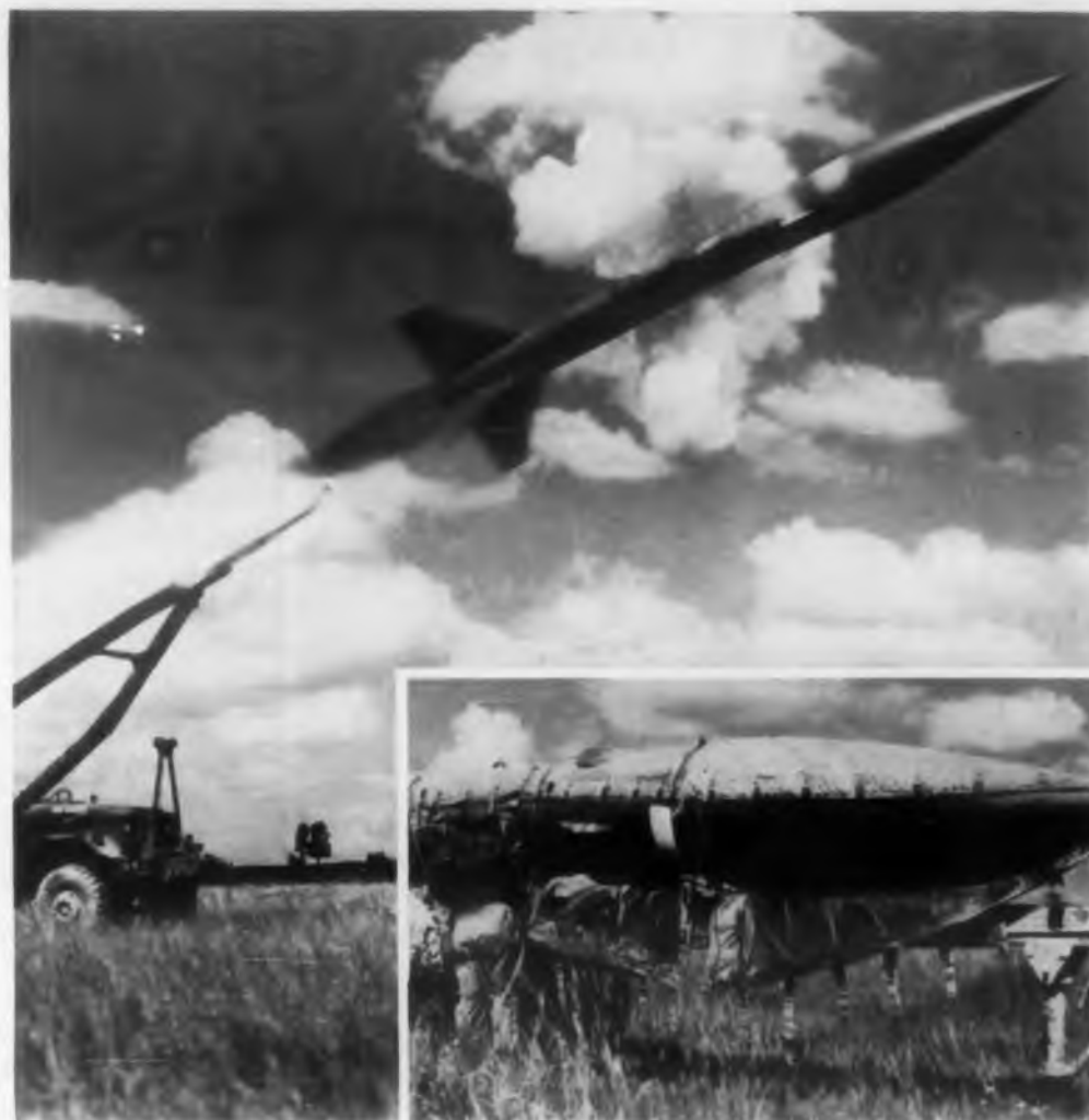
HONEST JOHN artillery rocket depends on G-E electric heating blanket (inset) to bring missile to uniform operating temperature before launching.
