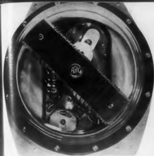
Loop antenna assembly of direction finder showing ferrite core mounted in housing.
