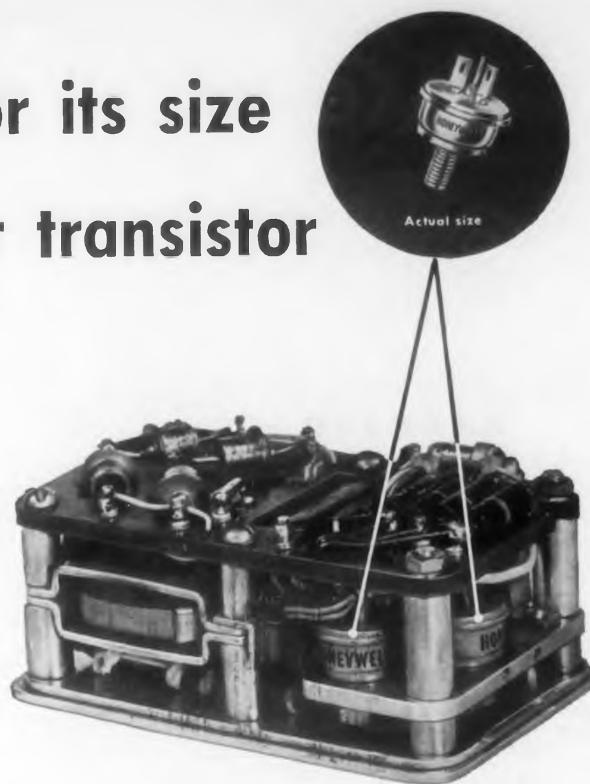
Honeywell stud-mounted 2N539 transistors make this 48-watt, 14 ounce D. C. Power Converter more compact than any other.
