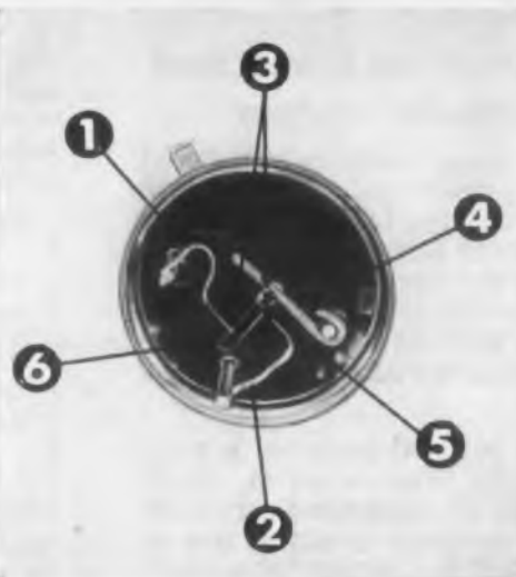
Photo shows top view of G-E silicon high-voltage transistor, with cap removed. 1. Gold emitter ribbon. 2. Aluminum base-lead ribbon. 3. Gold-silicon alloy. 4. Collector tab. 5. Base region. 6. NPN diffused meltback silicon bar. Cantilever design for shock resistance. Silicon bar is alloyed firmly to tab; ribbons are flexible to minimize constraints.
