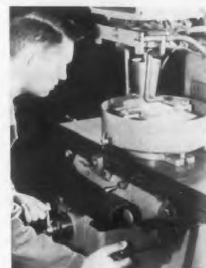
Fig. 1. Getting ready to "machine" semiconductor wafers by ultrasonics.
