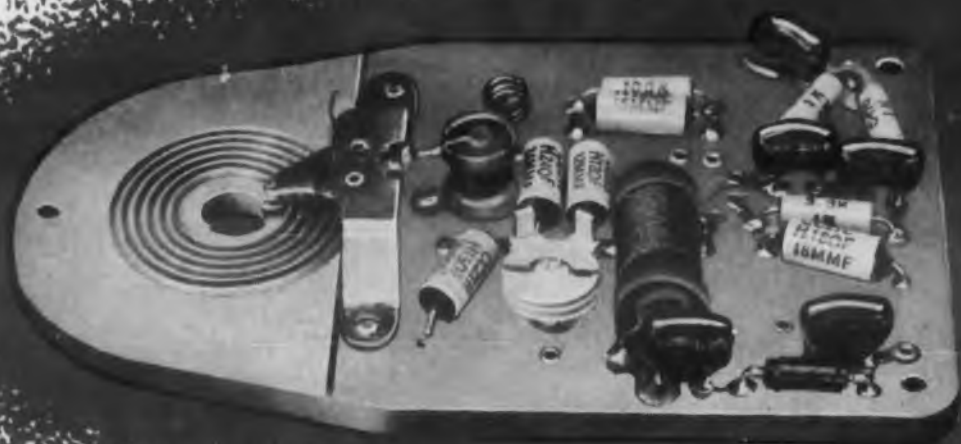
OSCILLATOR WITH SUPRAMICA 555 CERAMOPLASTIC BASE
