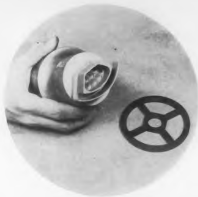
Fig. 3. Ferramic ring (right) produced by ultrasonic tool (left).
