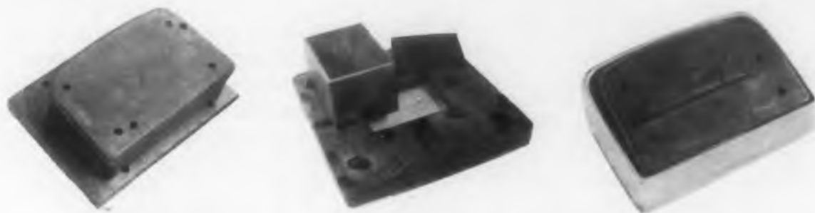
Basic Tooling for the cabinet shown on opposite page consists of a pressure plate, draw ring, and punch. Secondary tooling consists of a steel-sheathed masonite male and female pair for recessing the cover, which is drawn initially on the same die as the box.
