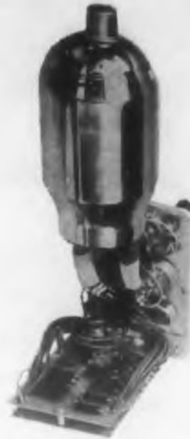
Fig. 1. Thermos bottle housing for transistor pairs. Transistors are mounted on an aluminum heat sink, potted with paraffin inside the thermos bottle. Temperature difference between transistors is negligible; total temperature rise due to enclosure is 5 F.
