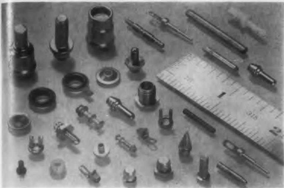
Fig. 2. Typical electronic and electrical "hardware" handled by the Freeloader. Items were manufactured by various methods—screw machine, stamping, molding and forming. Brass, steel, glass and plastic parts such as these are often small enough to require the use of tweezers with conventional assembly or processing methods.
