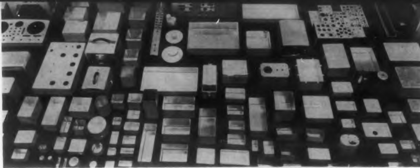
Versatility of deep-draw process is shown in the wide range of sizes, shapes and styles of enclosures, chassis, boxes, cans, and cabinets that have been produced.
