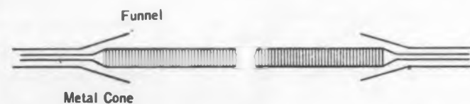
Fig. 2. Coupling scheme for coaxial system.
