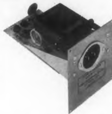
Fig. 2. Power supply construction. Supply is independent of line frequencies between 50 and 400 cy.
