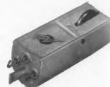
MODEL HS25-4 —Hermetically-sealed rocket safety switch, highly vibration resistant. Roller actuated. S.P.D.T., 1 circuit; 4 amps @ 30 V DC, res.; 2.5 amps., ind. Dimensions: 3\frac{3}{32} "x 1 "x 1 "
