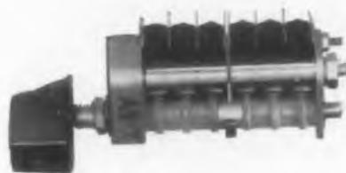
MODEL A9-7 —Multi-pole, ganged, sub-miniature assembly with rotary actuation. Positive detent-action gives exact indexing for accurate control. Dimensions: 3\frac{7}{32} "x 1\frac{1}{8} "x 2\frac{3}{32} "
