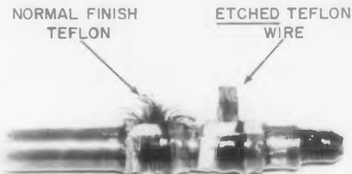
IMPREGNATED BOBBIN AFTER SLITTING COIL AXIALLY
