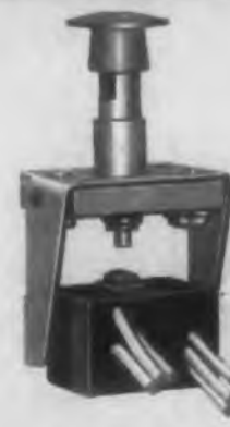
MODEL C3-8 —Vibration-free, positive detent-action, cut-off switch with potted wire leads in D.P.D.T. with simultaneous action. Dimensions: 1\frac{7}{8} "x 3\frac{3}{16} "x 1\frac{5}{8} "
