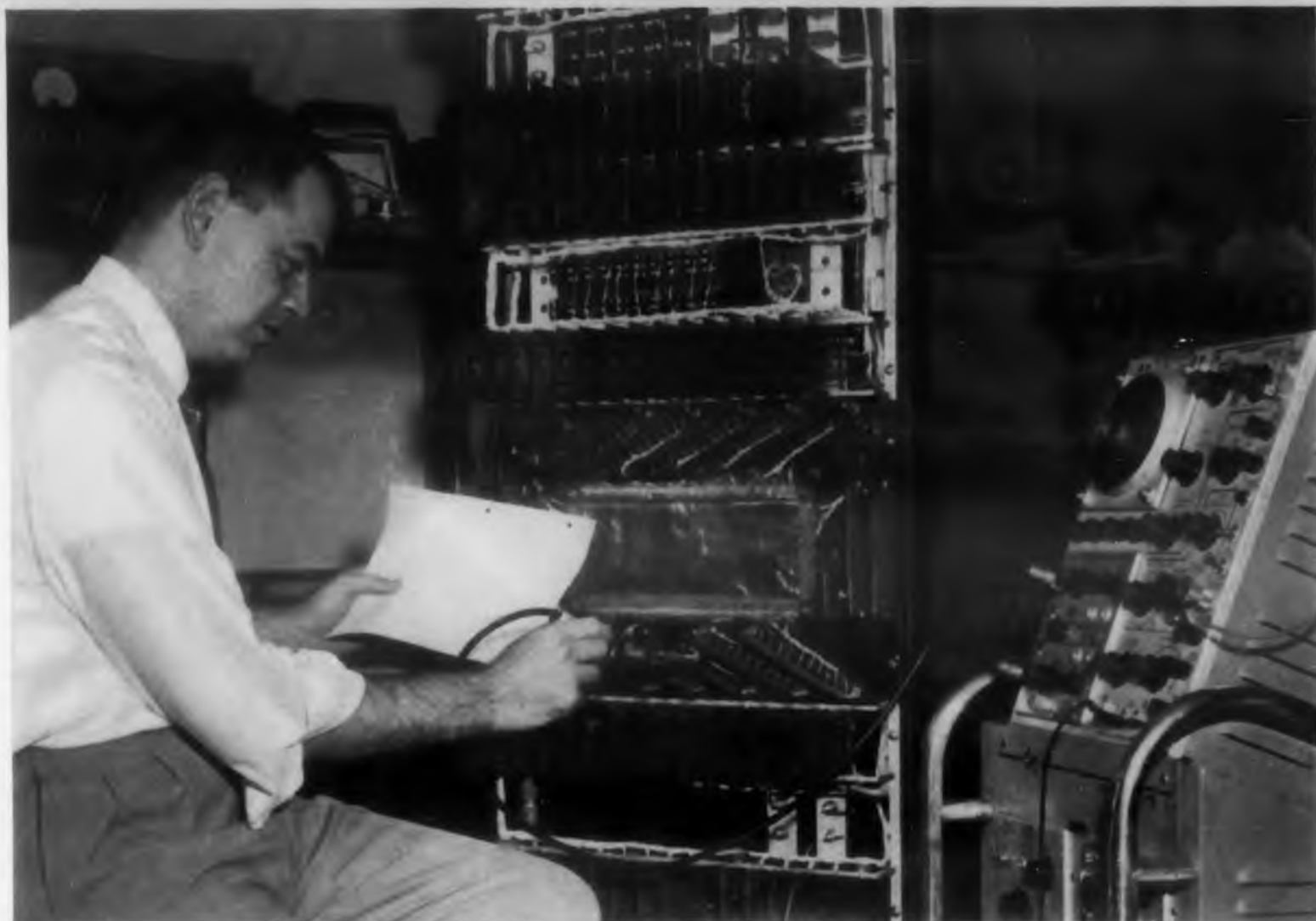
AN NCR ELECTRONIC ENGINEER checks the wave form of a transistorized magnetic core array tester.
