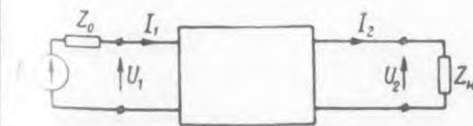
Fig. 3. Generalized four-terminal network. The following matrix equations apply:
