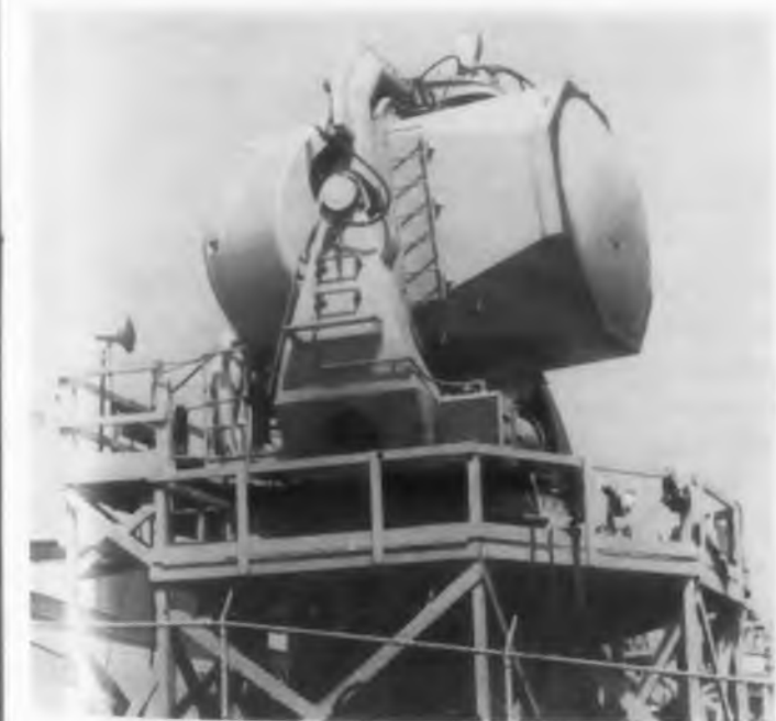
"Searchlight" antenna of Talos missile guides interceptors beyond the range of human sight.
