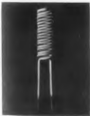
New heater uses straight tungsten wire
