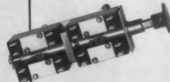
MODEL C3-13 —High current, manually-operated cut-off switch. Will simultaneously interrupt 4 circuits of 40 amps, 30 V. DC — or much higher voltages with lower amperages. Has 8 separate circuits available in one control device. Dimensions: 5\frac{1}{16} "x 1\frac{1}{2} "x 1\frac{1}{2} "
