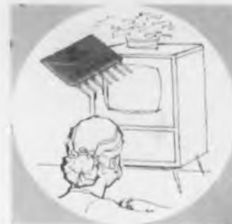
TV SETS—17 PEC's replaced over 100 parts, simplifying assembly and improving performance.
