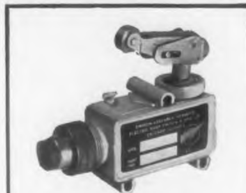
MODEL H1-43 —Stepless adjustment, roller-arm actuated, D.P.D.T. 4 circuit limit switch. Ribbed case hermetically sealed against heat and cold. Highly shock resistant. 10 amps @ 125/250 V. AC; 30 V. DC. Life 200,000 ops. Dimensions: 1 \frac{1}{4} " x 3 \frac{3}{4} " x 1 \frac{1}{2} " (Also available D.P.D.T.)
