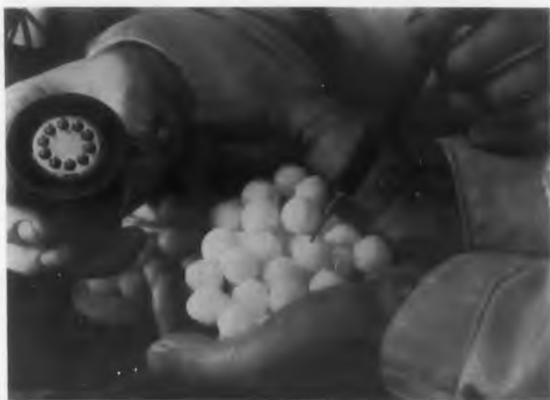
Mothballs (naphtalene) used as the organic compound which controls the gyro temperature.
