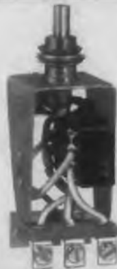
MODEL A9-6 —Rotary release switch. 2-position D.P.D.T., simultaneous action. Vibration resistant; binder screw termination. Dimensions: 1\frac{1}{4} "x 1\frac{1}{4} "x 3\frac{3}{16} "
