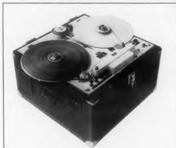
The "Magnetophon" German Tape Recorder—first high fidelity recording machine, subsequently improved and used to record and broadcast Bing Crosby's radio programs for over one year. The predecessor of all American Tape Recorders.
