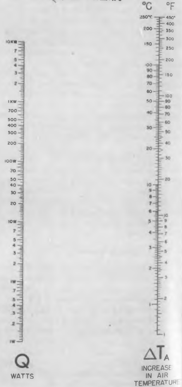
Fig. 6. Required air flow nomogram.
