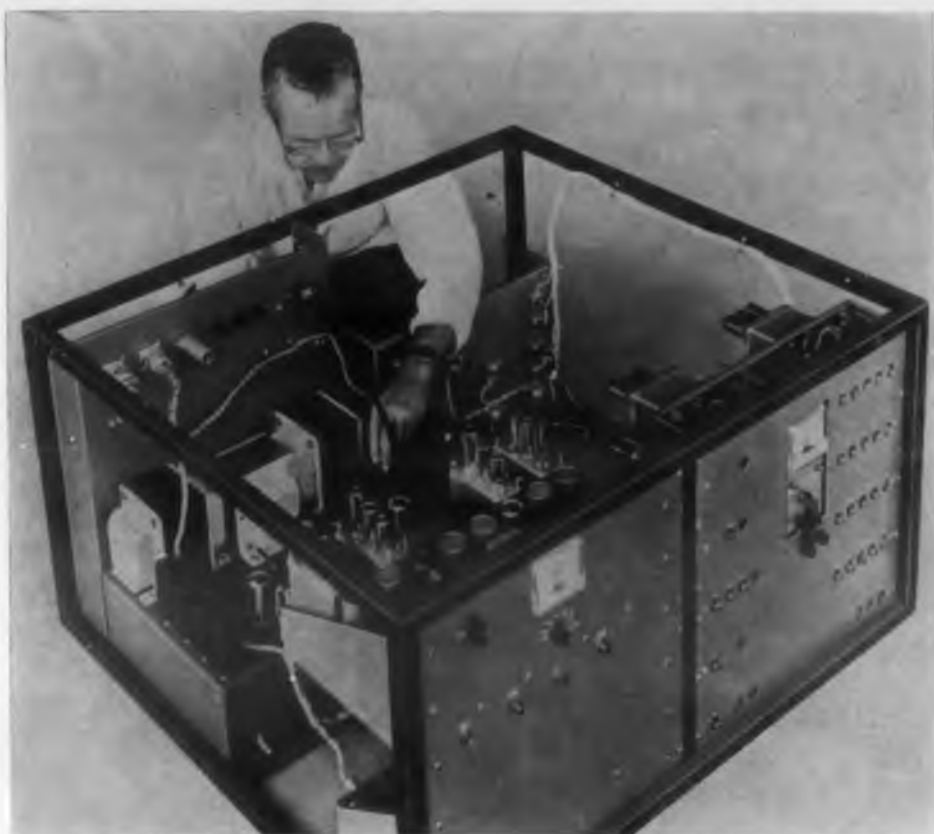
All electronic supplies, operational and servo amplifiers and servo networks are mounted in this rack.
