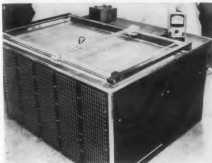
This electrolyte tank when connected to a computer, yields information on the operation of nuclear reactors.
