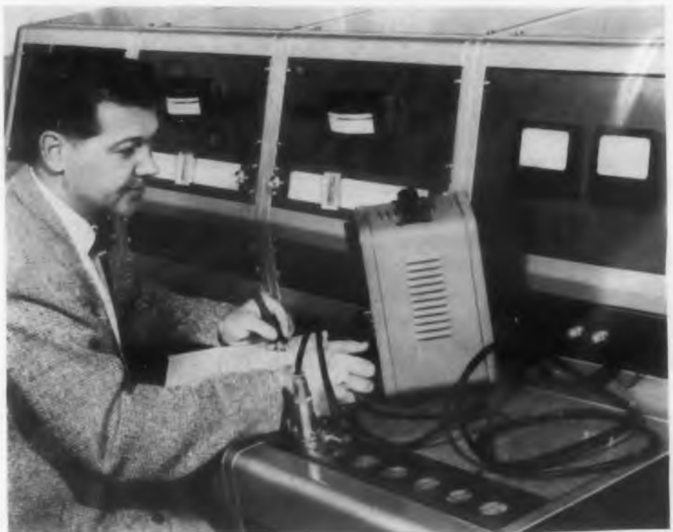
RF calibration consoles of the type used in the calibration of voltmeters.
