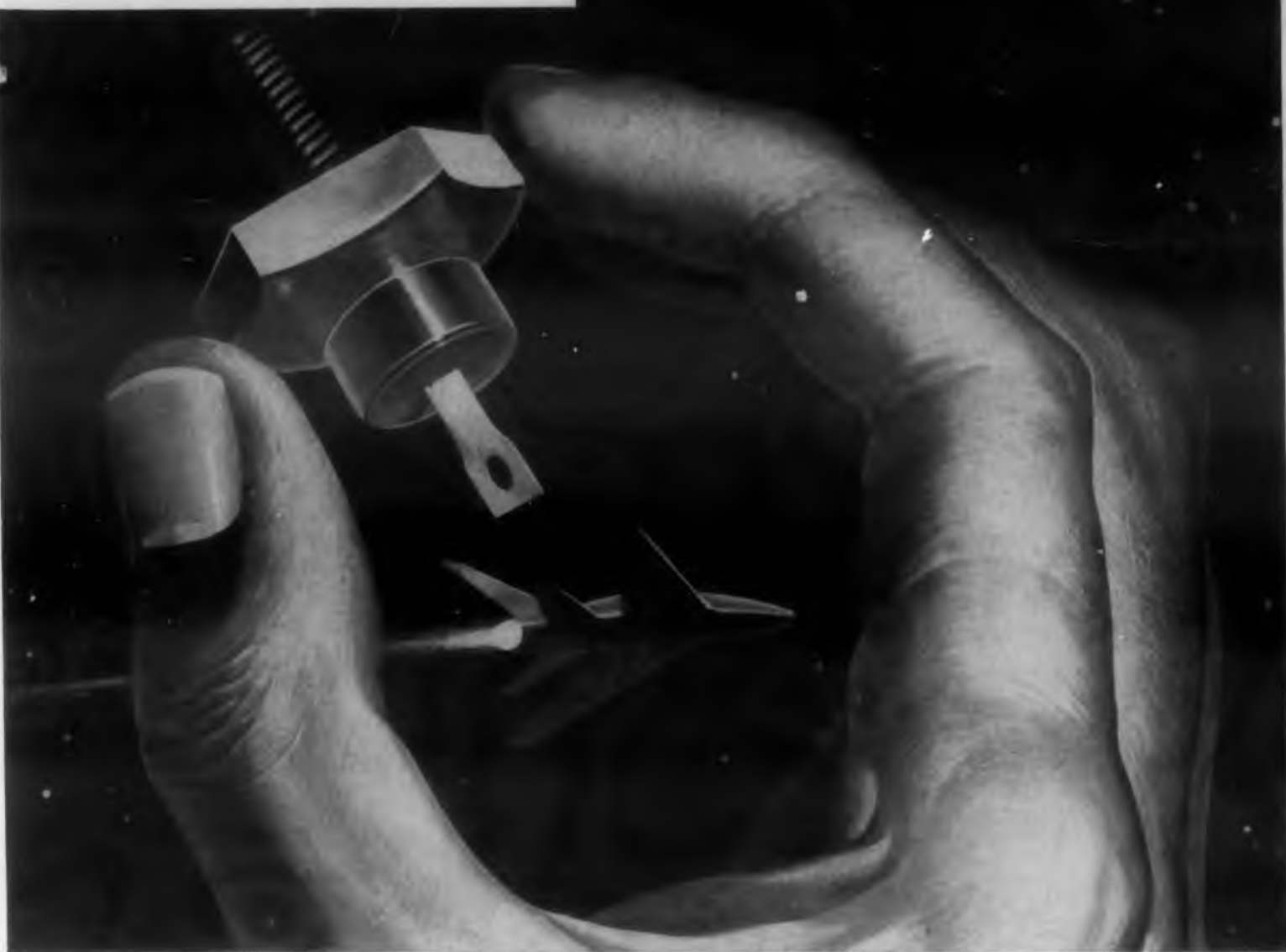
SILICON RECTIFIERS are finding increasing use at elevated temperatures in aircraft and missile applications by providing more power per pound.
