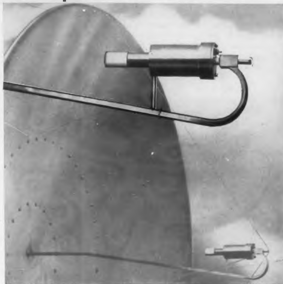
RADOME of a TEFLON resin matches impedance of feed horn to space and provides protection against weather. Wave-guide impedances at input and output of ferromagnetic
