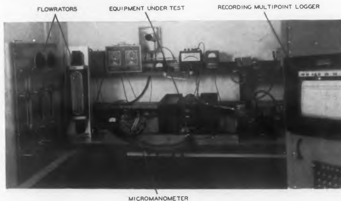
Fig. 1. Typical test equipment used for temperature and air flow measurements
