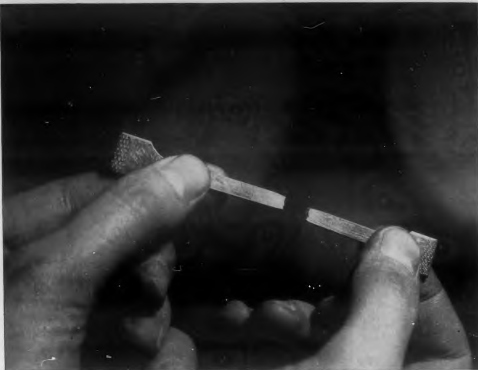
Elongation test of sample heelpiece metal typifies quality control measures that leave nothing to chance at Automatic Electric.
