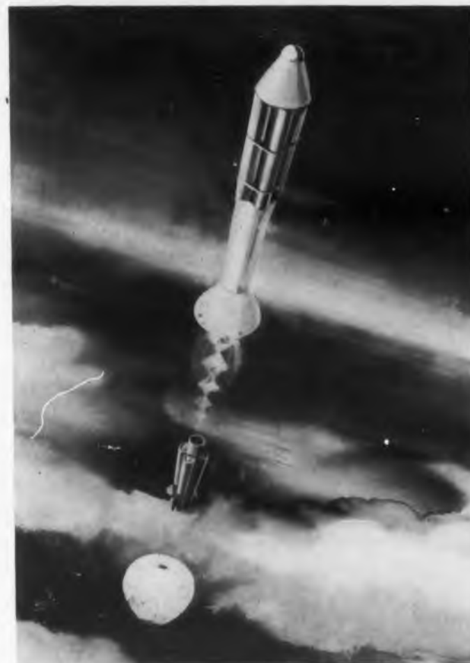
The rocket will be fired from its floating platform and will shoot up through the center of the supporting balloon.
