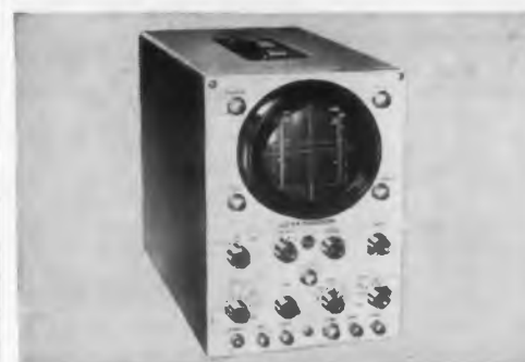
5" OSCILLOSCOPE WO-91A —Dual Band 4.5 Mc scope, for waveshape observation and measurement, signal tracing and alignment of chrominance circuits and wide-band amplifiers—voltage-calibrated input step-attenuators and calibrated graph screen make possible direct voltage readings as easily as with a VTVM. User Price $239.50*
