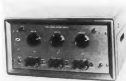
Two Phase Power Supply Total Output of 550 VA
