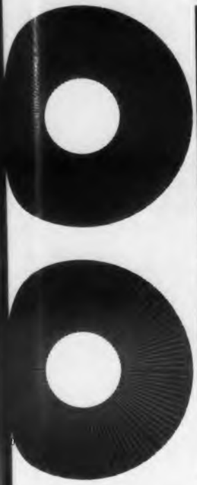
Fig. 1. The "printed" silver conductors of the rotor (top) and stator are etched on a glass disc.
