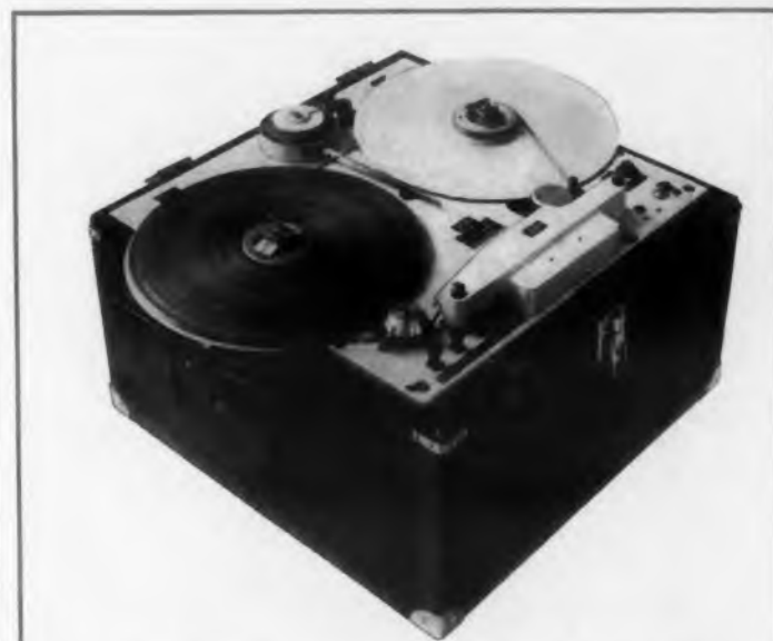
The "Magnetophon" German Tape Recorder—first high fidelity recording machine, subsequently improved and used to record and broadcast Bing Crosby's radio programs for over one year. The predecessor of all American Tape Recorders.
