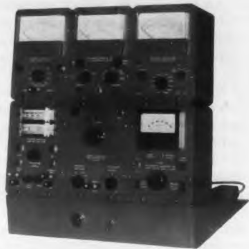
Fig. 2 Instruments can be simply stacked upon one another. For semi-permanent installations, a locking strip and stand are available.
