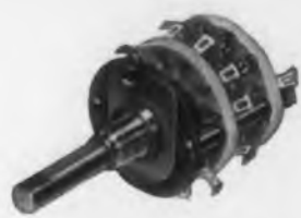
Type F: Miniature 12-position, 30-60° throw, can be mounted in 1-5/16" circle; phenolic, Mycalex or steatite.
