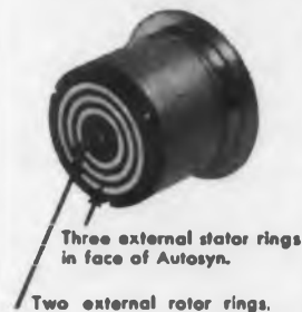
Rotor and stator rings mounted concentrically with outside diameter of housing. Rotatable gear mounted to Autosyn.
