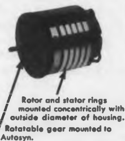
Three external stator rings in face of Autosyn. Two external rotor rings.
