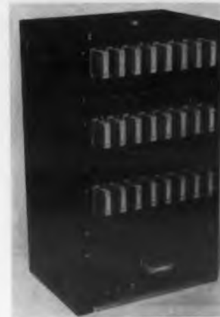
Dry Circuit Tester Checks Relays
