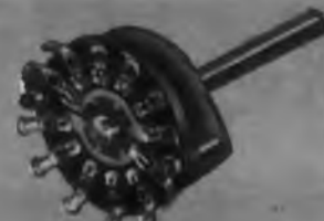
Type H: Standard 12-position; 1-7/8" diameter; 15-30-60° throw; phenolic, Mycalex or steatite.
