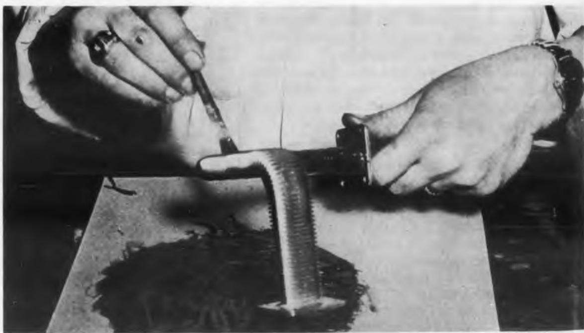
Rigidizing compound is brushed on flexible waveguide. Complicated assemblies can be easily fabricated using this technique.
