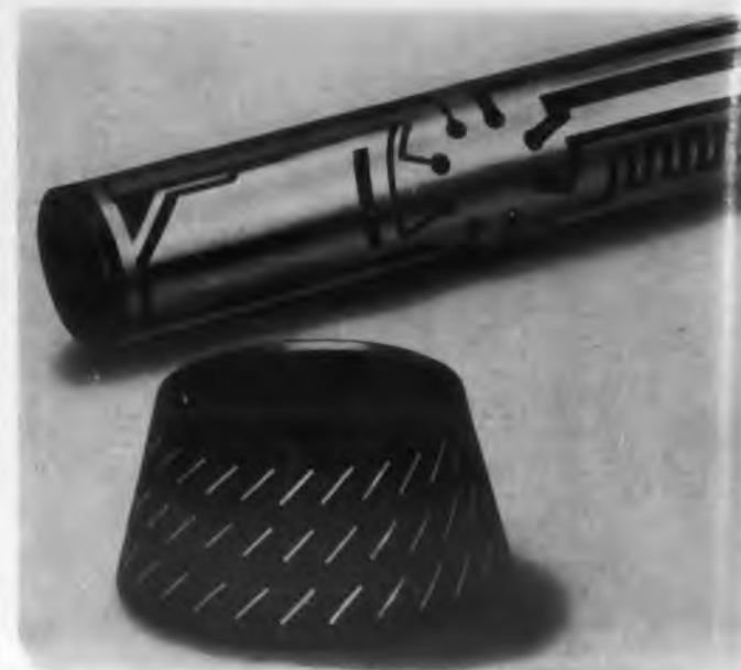
Fig. 1. Direct-printed circuits on cylindrical and conical surfaces. Circuits can be printed inside or on both sides of tube. The truncated cone is a depolarizing element of a discone-type antenna.
