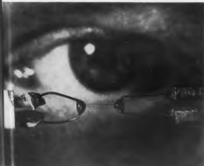
Interatomic forces in an iron crystal "whisker" are measured by stretching the tiny strand of metal.
