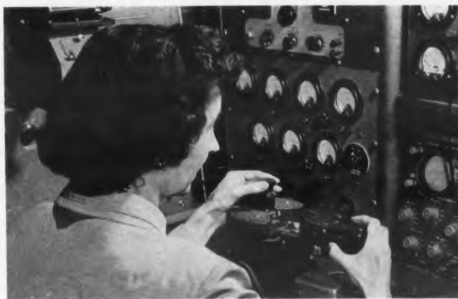
Fig. 3. An operator is sliding a subminiature tube into the exciter block in preparation for a vibration test. Tube leads are held in a clamping device which connects the tube to its operating circuit during test.
