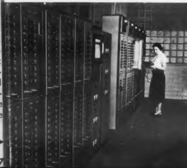
Shown below is a portion of the Life Test Section where all types of Philco transistors are tested under a variety of storage and operational conditions. Individual test positions are provided for over 10,000 units.
