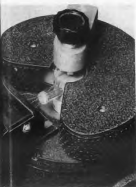
Fig. 2. Closeup of the vibration exciter shows the tube envelope secured in a block on the exciter table.
