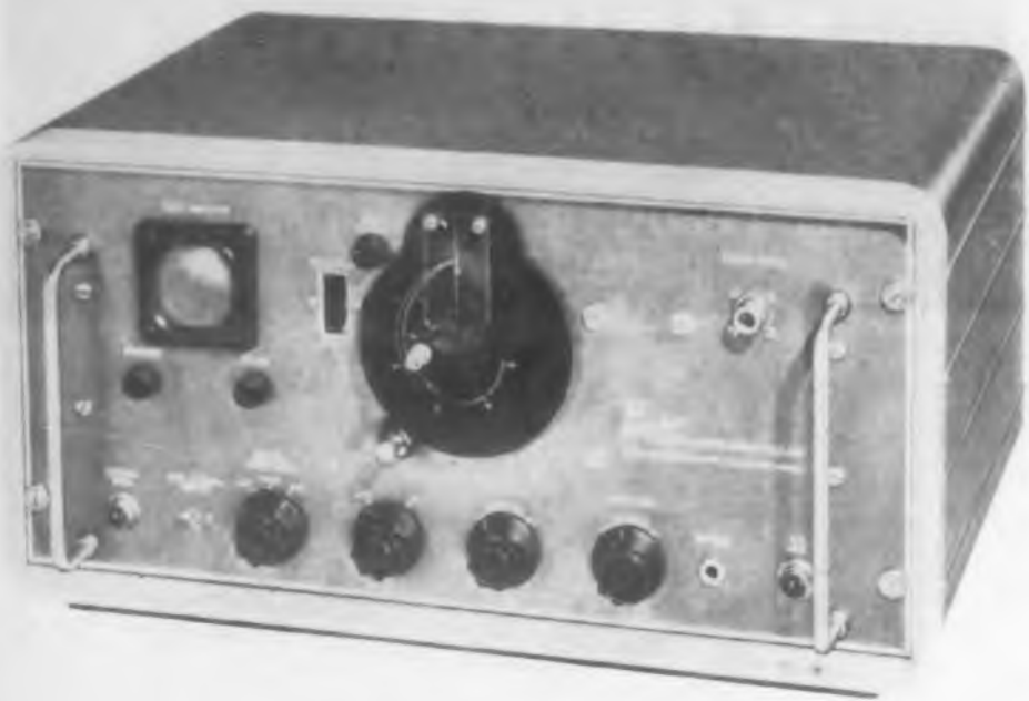
Fig. 1. Automatic Interpolation dial in use on PRD Type 504 Heterodyne Frequency Meter.
