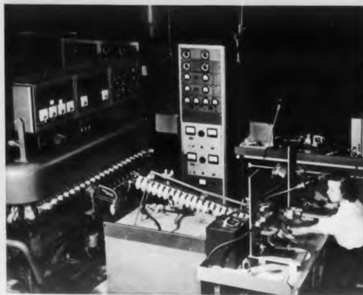
New Philco automatic "Carousel" assembles and processes alloy junction type transistors. It prepares stems by localized plating, solders stems to transistors, solders leads to emitters and collectors, and follows with electrolytic clean-up etching, dip rinsing and ultra sonic rinsing to remove contaminants.
