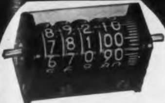
High speed, non-reset, direct reading counter to indicate increment of measurement in radar navigation instruments.
