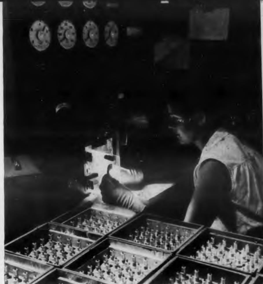
GL-6442 triodes are individually tested for their electrical characteristics, in order to assure tube dependability and full-rating performance at all times.
