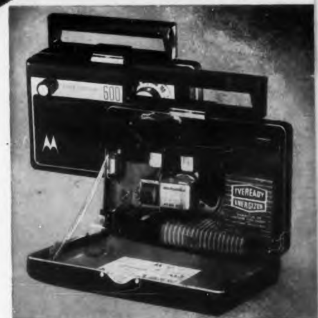
The Motorola "Ranger" achieves compact, sturdy construction and fast assembly with plated circuits on laminated stock produced by Farley & Loetscher Mfg. Co., Dubuque, Iowa, using BAKELITE Laminating Varnishes.
