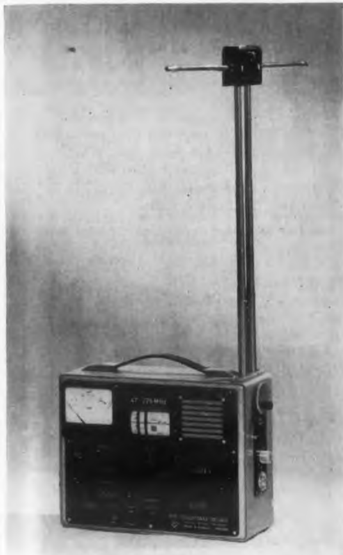
Portable vhf field strength meter covers vhf broadcasting, TV, aircraft and police radio frequencies.
