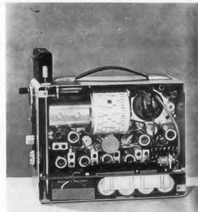
Vhf field strength meter consists of a superheterodyne am-fm receiver, a dial calibrating oscillator and dry battery power supply.
