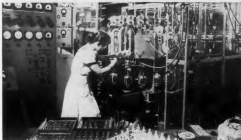
The tubes are evacuated by rotary exhaust machine; afterwards, their metal stems are pinched off and sealed.
