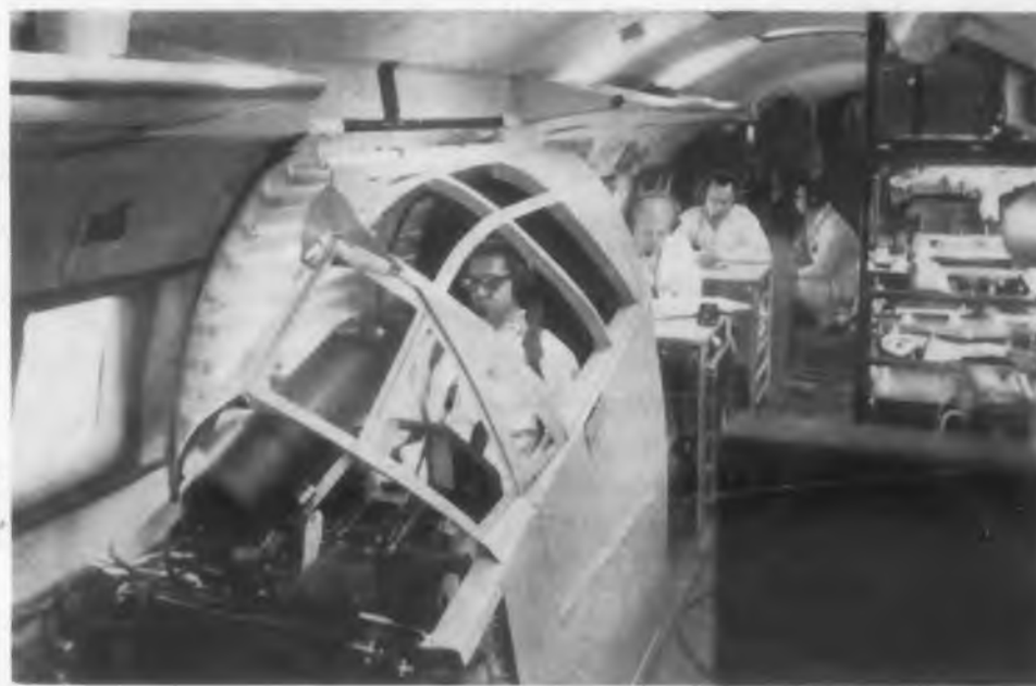
In a cockpit installed in the main cabin of a T-29 airliner, a second pilot takes over control of the plane once the regular pilot has taken it aloft. At left is a layout of the flying laboratory.
