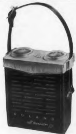
Compact small portable is illustrated well by Roland's all-transistor 66. Four-in. speaker is larger than most.
