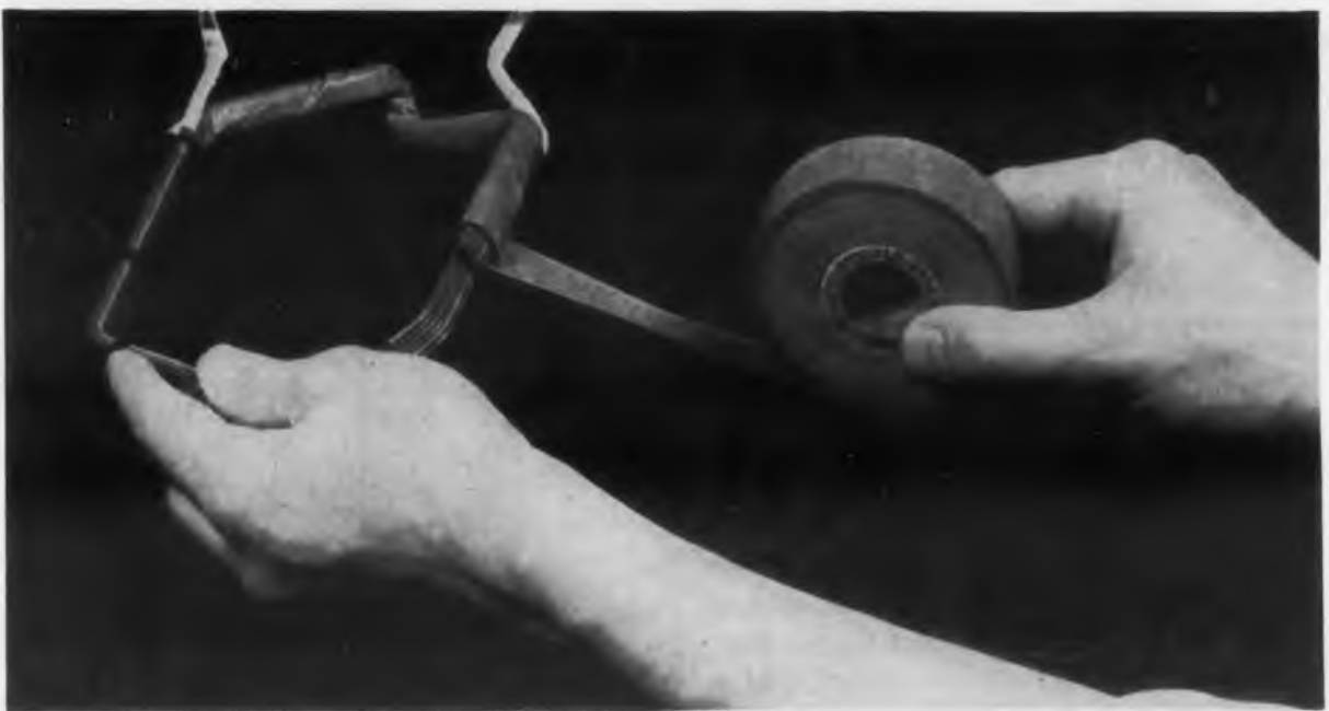
Shown here is epoxy-resin tape X-1045—a non-woven polyester mat impregnated with epoxy resin—being applied to a motor coil. The fully wrapped coil is cured and pressed to provide a smooth hard surface which is shaped to fit snugly in its slots.
