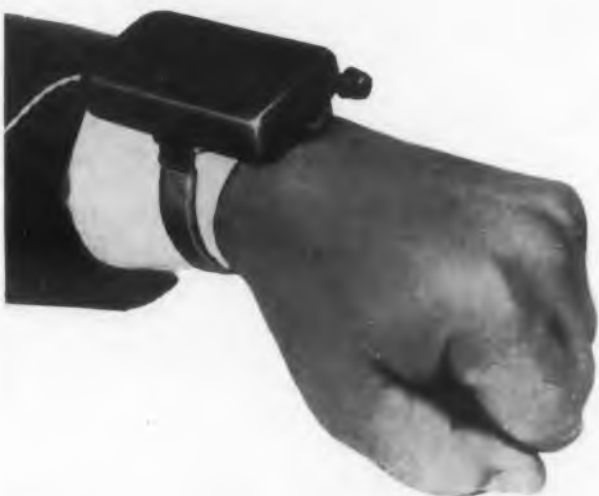
Wrist model (somewhat king-sized) of LEL, Co-piague, N. Y. uses regenerative circuit.
