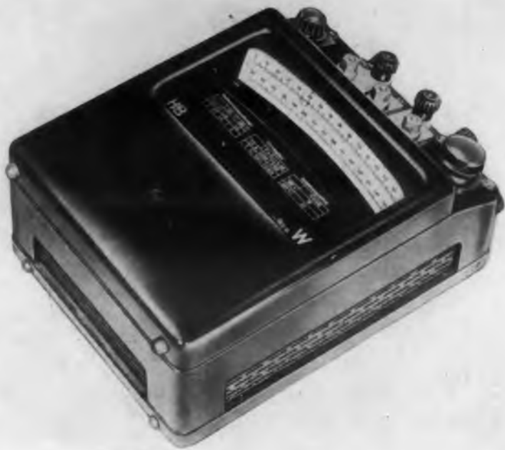
Fig. 8. Light Spot Watt Meter. This Hartmann and Braun design eliminates the needle pointer common to galvanometer type instruments. Several interesting advantages result. By focusing a light spot onto a mirror affixed to the moving coil, scale illumination follows coil movement. No external illumination is necessary to read the meter. An important feature is that there is no parallax since the cross-hair in the light beam appears directly on the scale. Meter sensitivity can be greater because less force is necessary to move the coil than when a needle pointer is attached. Also, there is no mechanical damage to the instrument on overload. The light beam will move off scale but there is no needle to "wrap around the pin."
