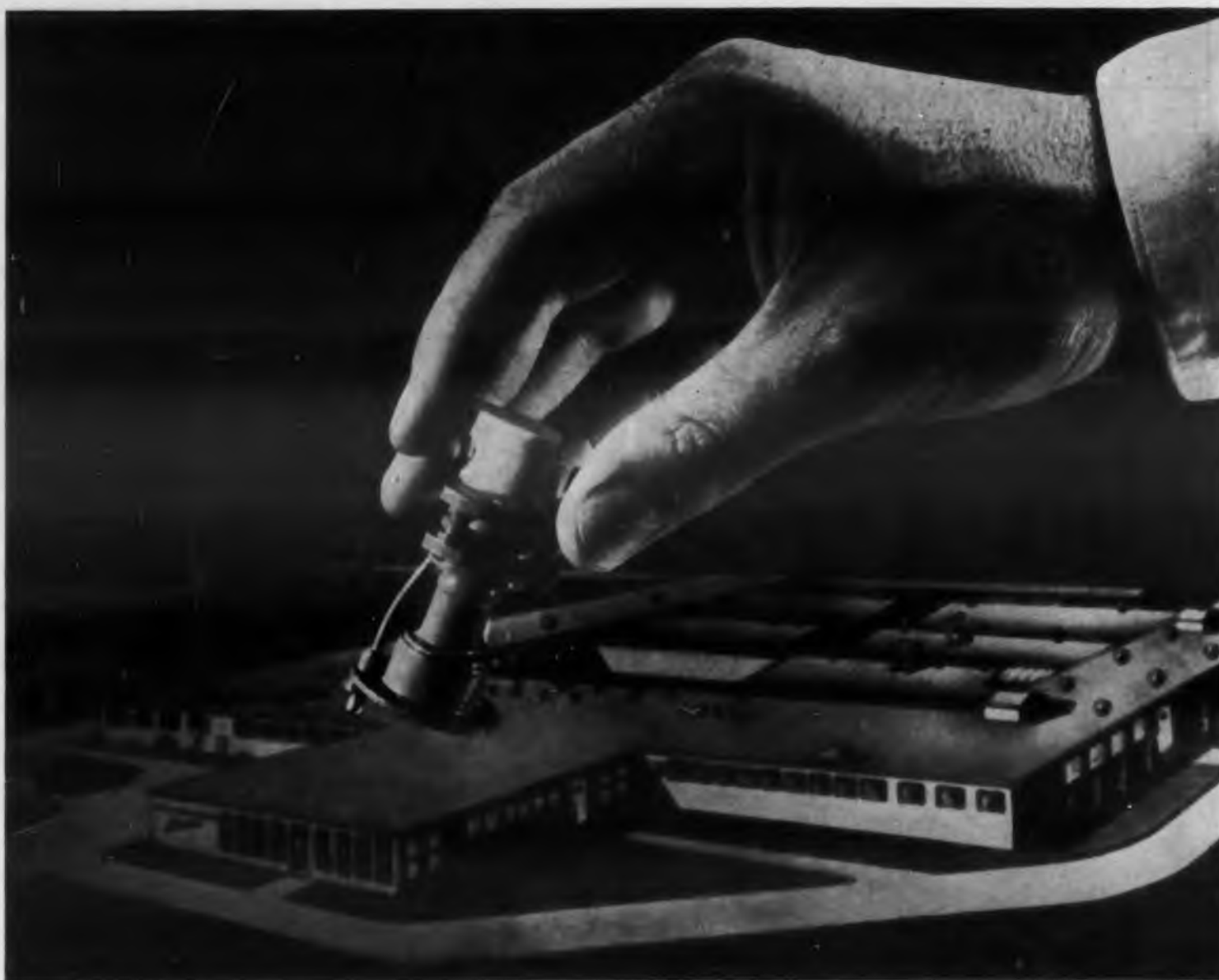
Hand holds Eimac 1K015CA local oscillator C Band Klystron, 5300-6000 MC
