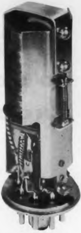
Fig. C Plug-in type high-sensitivity relay with cover removed.
