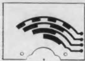
Fig. C. An example of one possible form of a typical printed-circuit dial plate.
