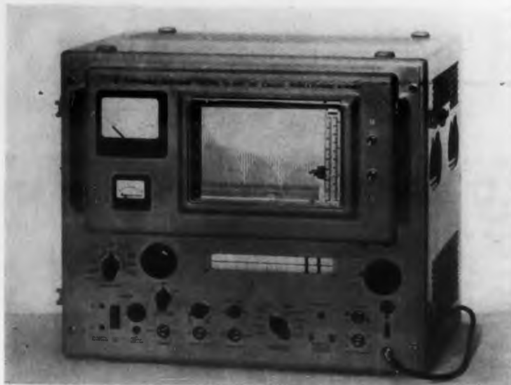
Fig. 6. Audio Frequency Spectrograph. This instrument analyzes the spectrum, from 20cy to 20kc. Unusually high resolution is provided, with selectivity of 10cy or 200cy available as desired. An 80db signal difference can be detected. An especially interesting feature is the method of data presentation. Graph paper can be inserted from the top of the chart frame provided and readily removed from the bottom by pushing appropriate buttons on the panel. An ink recorder automatically traces the pattern over any selected 5kc band.
