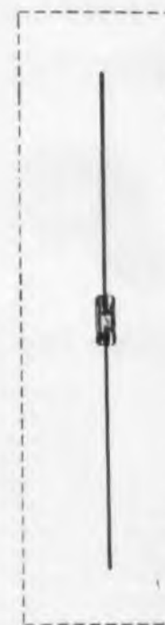
*Actual size, diode body: 0.265 by 0.130 inches, maximum.
