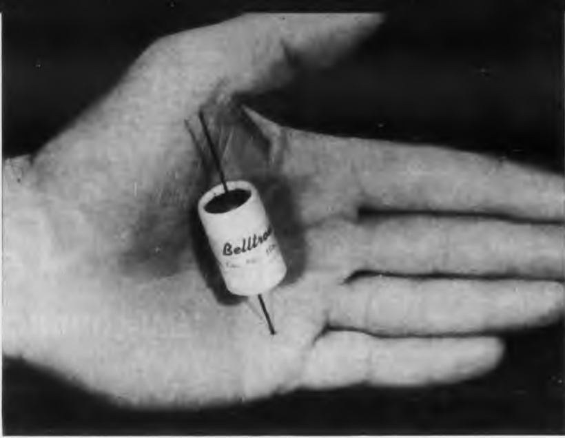
Fig. 1. This miniature relay furnishes a wide range of specified time delays.
