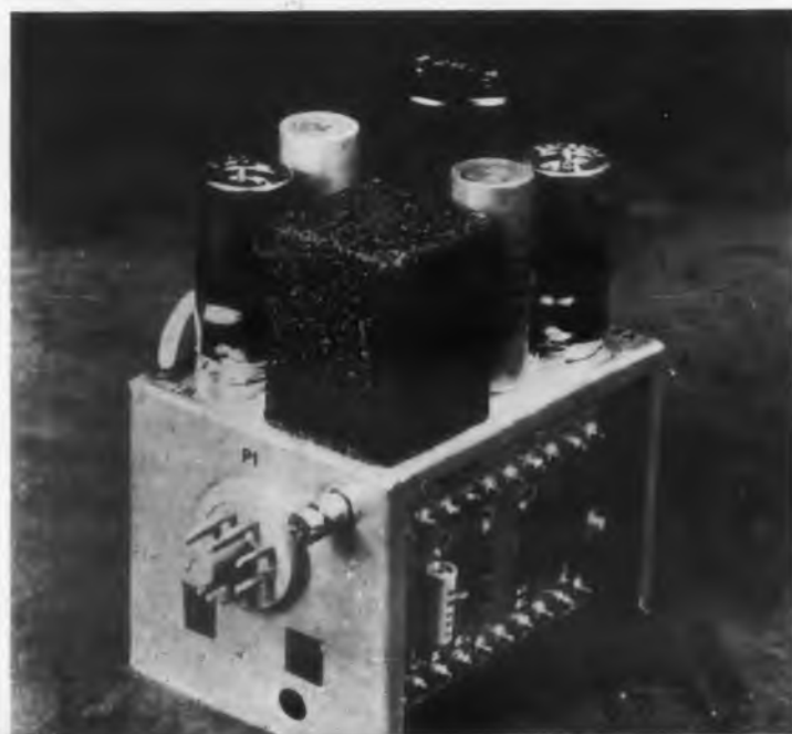
Fig. 3. Weighing only 2 lb, the linear phase detector is 3-1/8" x 4" x 5-1/2" high including tubes.
