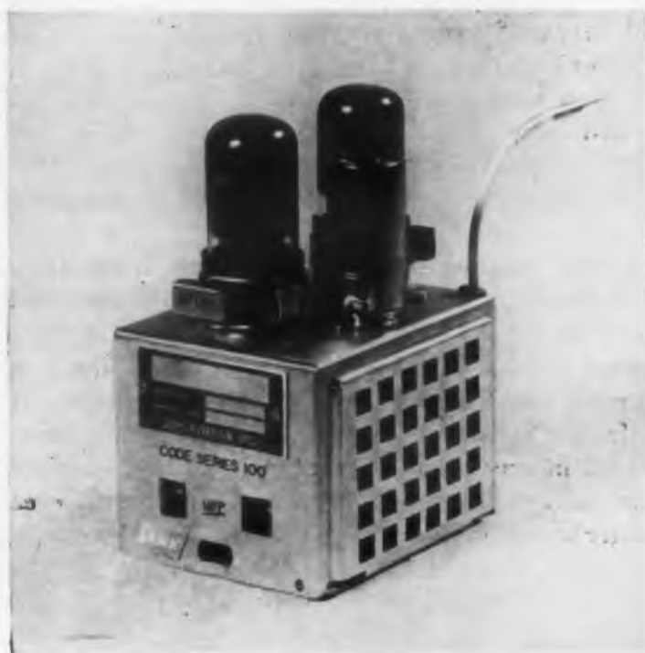
Fig. 2. The servo amplifier is 3" x 3-1/8" x 6" high including tubes and weighs 1-1/4 lb.
