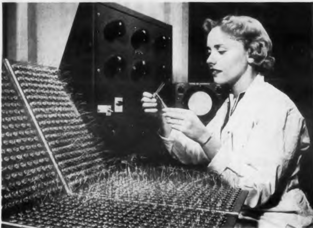
Transistor uniformity and high performance are assured with the constant temperature, humidity and dust-free conditions provided for our production line.
