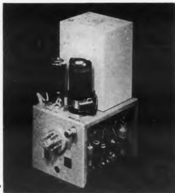
Fig. 5. The summing amplifier has a power output of 3w. It is 3-1/8" x 4" x 7" high with tubes in place and weighs 4 lb.
