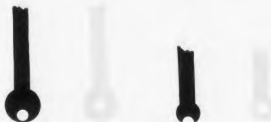
Fig. 3. The possible results of making a termination too small is shown at the right in black. At the left, the same misregistration of the hole punch still leaves a usable termination.
