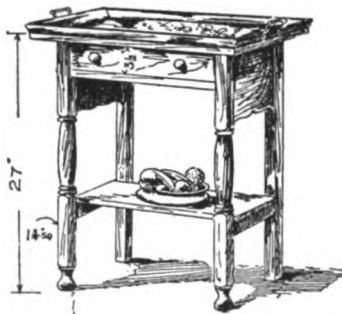
Fig. 7—A Tray Table to Fit Glass Tray 10 x 25 In.
