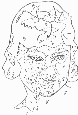
Fig. 3. This is Part of the Program or Code Telegraphic Message—the Form in Which the Picture is Flashed Over the Wires.
