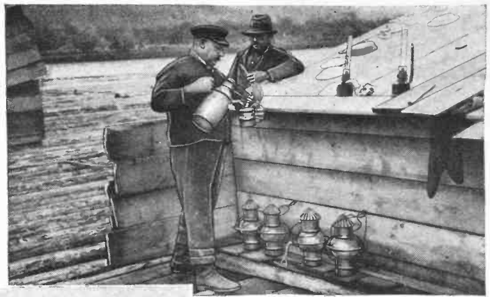
Filling oil lamps for the night on the Rhine. Running lights mark the position and extent of the raft for the guidance of other craft navigating the river at night.
