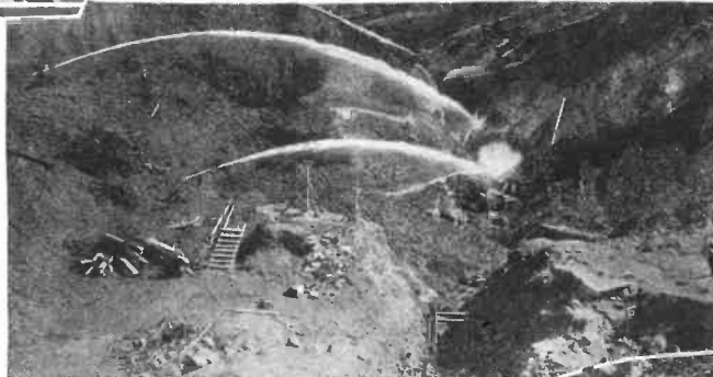
Native labor sluicing for gold at Edie Creek, in the uttermost wilds of New Guinea. High power hoses wash away the earth, and the free gold is left in settling pans. The native boys are paid $1.50 per month. Not the least of the many dangers encountered in this region is cannibals.
