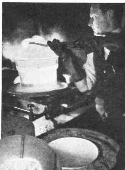
Testing glass insulators, the glass is chilled to -98^{\circ} C. and then dipped in to boiling water. Below—An insulator under breakdown test.
