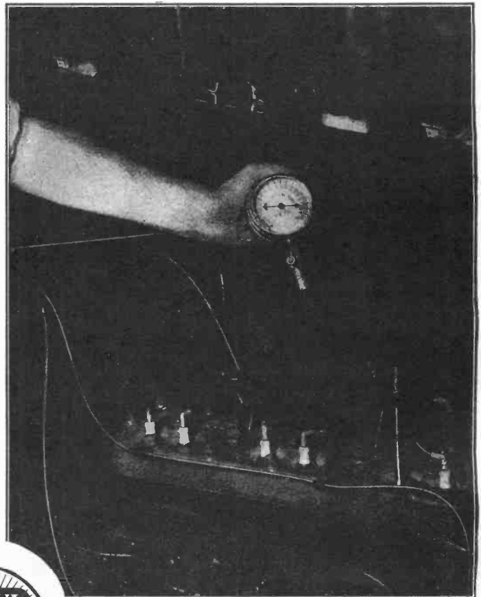
Taking the compression pressure of a stock model car with special head. 175 pounds compression is a much higher pressure than that of any car on the market, and this engine is operating satisfactorily on Ethyl Gasoline.
