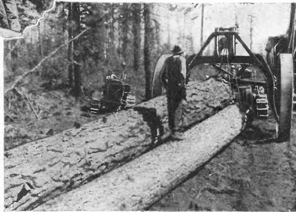
Top, left—The purpose of this "undercut" is to direct the fall of the tree so that it will not damage its own and other trunks and thus waste valuable timber. After the undercut is made, sawing begins on the opposite side, wedges being driven in back of the saw to keep it from binding. Above—Caterpillar Sixty with high wheeler and fair lead, hauling timber to water.
