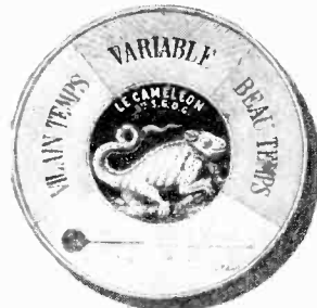
The Chameleon Barometer is a chemical hygroscope using a cobalt salt, which changes color from blue to pink with increase of atmospheric moisture. The significance of the colors is shown by three tinted sectors in the margin.
