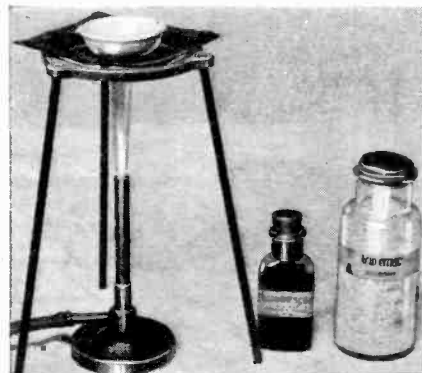
Preparing a fused mixture of fluorescein and citric acid in air-evaporating dish. This mixture gives bright phosphorescence.
