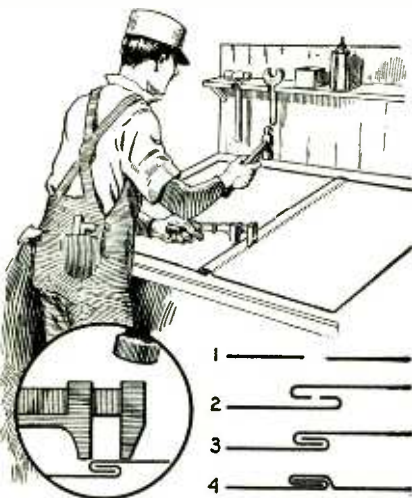
The drawing shows the four successive stages in making a lock joint between two pieces of sheet metal in the manner here described. First the edges of the two sheets are bent to the shapes shown at figure 2; next these two bent edges are interlocked as shown at figure 3. Finally the joint is locked as in figure 4, by simply holding the wrench over the ridge of metal formed by the juncture of the two folded bends, and repeatedly striking the wrench with a hammer as the man in the picture is shown doing.
