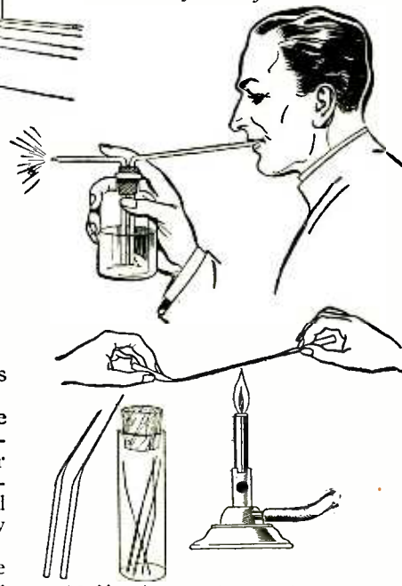
Making burette cleaners from glass tubing.
