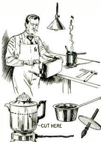
Remove handle of percolator and cut at dotted line; make glue pot with flat rim that extends over side of percolator.
