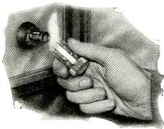
The above photograph shows the automobile cigarette lighter in operation. The cover is pulled off to light the device.
