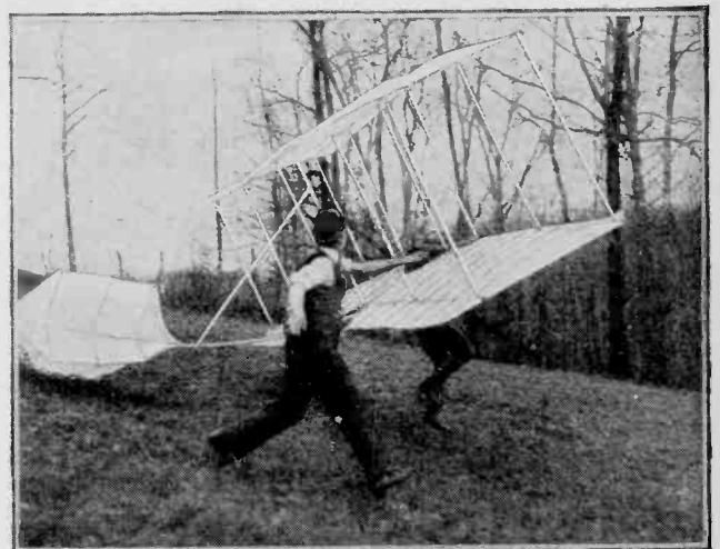
Fig. 6—When landing, the wings are tilted sharply, so as to offer a greater resistance to the air, as shown above.
