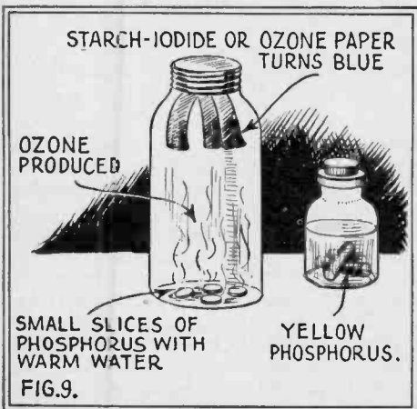
FIG. 9. To test for ozone, a special "ozone paper" is needed. When exposed to ozone, the test paper will turn blue.
