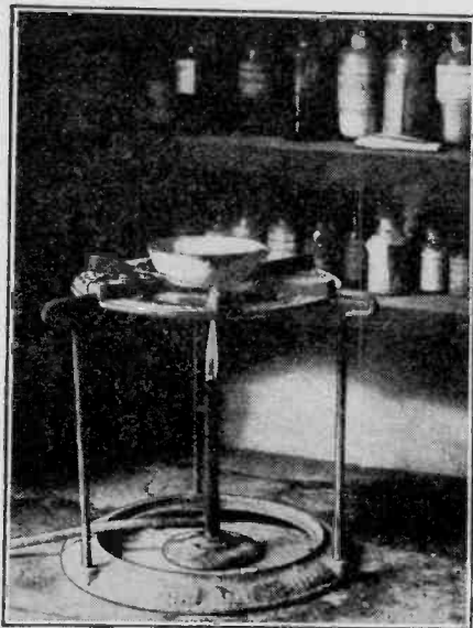
The above photograph shows how the glycerine is dehydrated in a porcelain dish over a small flame. About 35 c.c. of this substance is used in the experiment.
