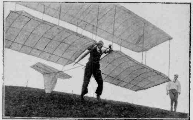
Fig. 3—The above photograph shows the glider just after it has been released by the assistants. When the pilot feels the plane pulling upward, he signals to be let free.
