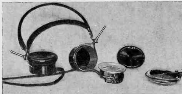
The materials used in making an electrical phonograph pick-up appear above. An old Columbia reproducer and Baldwin type C headphones are used. Except for cutting a few pieces of brass the construction is an assembly.
