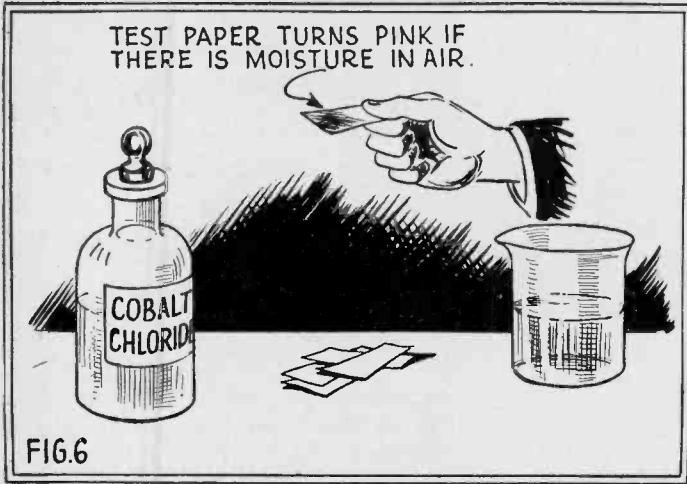
FIG. 6 A strip of paper moistened with cobalt chloride when thoroughly dried will be almost colorless. When exposed to moist air, it turns pink.
