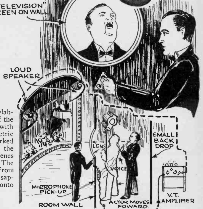
In one of the scenes, a pair of hands are observed playing on a piano keyboard in a vertical position through a "television" window. How this mystical scene is staged is clearly shown above. Scene at right shows how face is made to grow larger in "television" screen.
