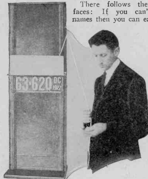
Fig. 7. This is a front view of the device illustrated in Fig. 6. The shutter arrangement permits of a two second observation period.
