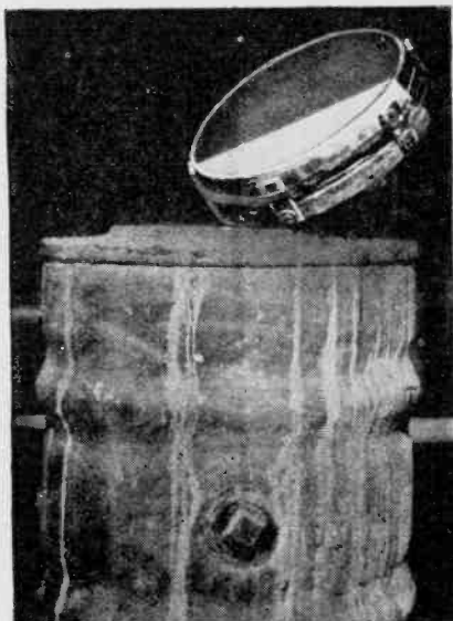
The photograph above shows the mirror, tool and grinding post at the completion of the fine grinding. The tool is cemented to the top of the oil drum.
