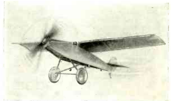
A flying model of an airplane with demountable wings driven by a rubber band motor and capable of actual flight is shown above.
