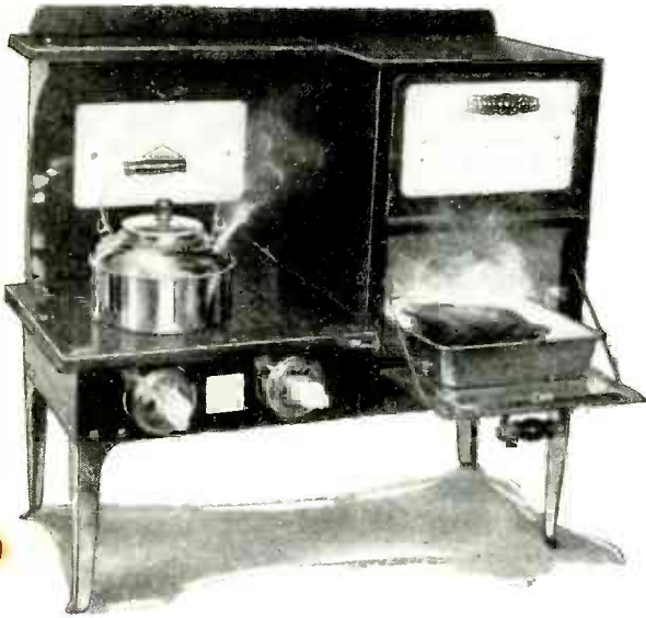
A small electric stove similar to a gas range is shown above. Electric heating coils are used for cooking the food. The switch at the left controls the current supply to the outside cooker, and the right-hand switch controls the heating coils in the oven and broiler. The illustration at the left shows the placement of heating coils and grids. The model is of sturdy metal construction and is finished in black and white enamel, similar to large stoves.
