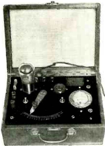
The above photograph shows a manufactured A.C. and D.C. tube tester and rejuvenator. The pointer is varied to obtain different filament voltages.
