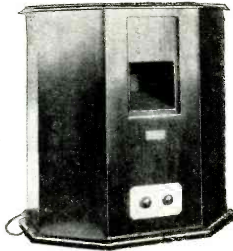
The photograph shows a view of one of the first complete manufactured television receivers. It is contained in a walnut cabinet measuring 26 in. x 26 in. x 13 in.
