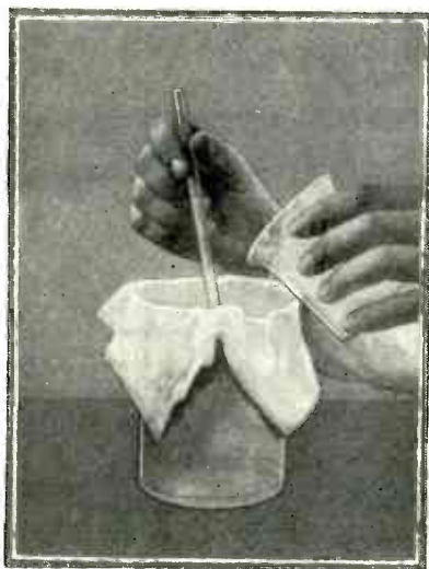
Above—filtering off the soap through a piece of fine cloth. Cheese cloth may be used for the purpose.
