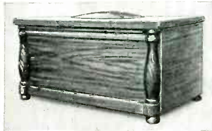
The finished chest as seen from the front appears above. If close grained wood is used, an on-rubbed finish is suggested and an oil finish with open grained wood.
