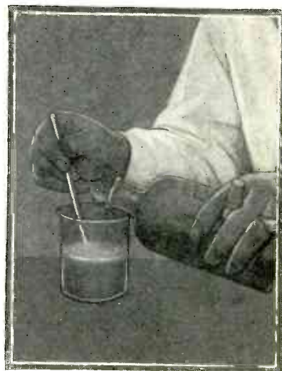
Free lauric acid which floats on top of the water can be obtained by dissolving the soap in water and adding hydrochloric acid. Lauric acid is found in cocoonut oil.
