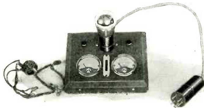
A new A.C. tube and set tester appears in the above photo. All types of A.C. tubes can be used in this instrument. A harness is provided for testing those tubes having cathode connected to one side of the heater element.
