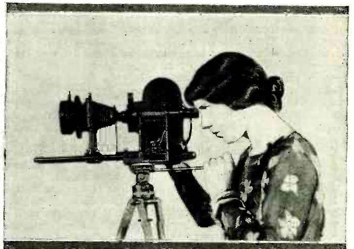
The new effect set complete and in use is shown above. Note the special mounting which permits the camera to be adjusted by a handle which allows any vertical or horizontal position.
