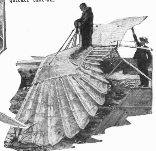
The wing spread of the ornithopter is 29½ feet. Note how bird-like the ends of the wings are, as tipped with feather-like constructions. Photo was taken on the beach at St. Augustine, Fla., where the first test is to be made.
