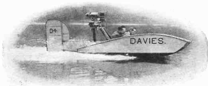
Powered only with a motorcycle engine and driven by an air screw, this hydro-glider was able to make a speed of 30 miles an hour on the river Severn in England. Photo shows glider running up stream.
