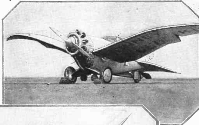
The above photograph shows the "Bonny Gull" poised for flight. The wing angle could be changed to permit of quicker take-off.
