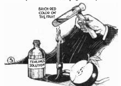
Fehling's solution is a delicate test for fruit sugar and will show the presence of a minute quantity of this nutrient by the formation of a brick-red precipitate.
