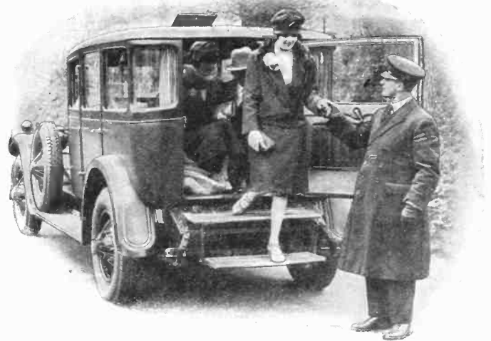
The new tourist body for automobiles is shown in the photograph above. The back of the car represents an observation platform.
