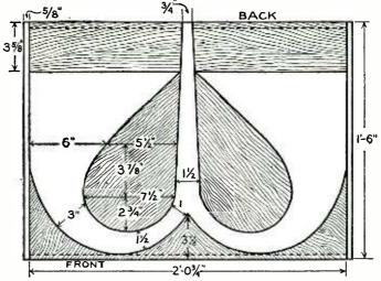
A section of the central part of a folded exponential horn is given above. The entire section is  $1\frac{1}{2}$  inches thick and fits into the central Section, which is shown below. This horn has a cut-off frequency of 128 cycles.
