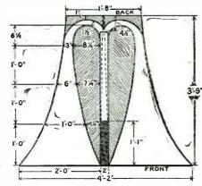
Plan layout of baseboard and central section of the 12-foot horn is given above.
