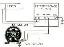
The wiring diagram of the radio interference filter is given above. The manufacturer of this device makes a small filter for use with equipment rated up to one-quarter horse-power, and a large filter to be used with motors and other appliances up to 5 horse-power at 220 volts. Five terminals are pro-vided on the filter.
