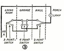
Any number of points of control may be added by connecting four-point switches between the two three-point switches, as shown above in Fig. 3 for garage use.
