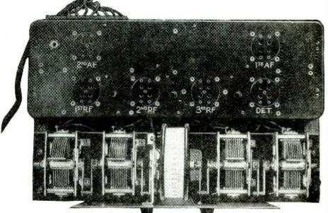
The chassis of the new receiver is shown here. The four tuning condensers are arranged for drurn control. Another novel feature lies in the fact that the illuminated dial is calibrated in wave-lengths. (Name of manufacturer furnished upon request.)
