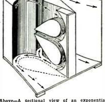
Above—A sectional view of an exponential horn folded into a small compass is shown above.
