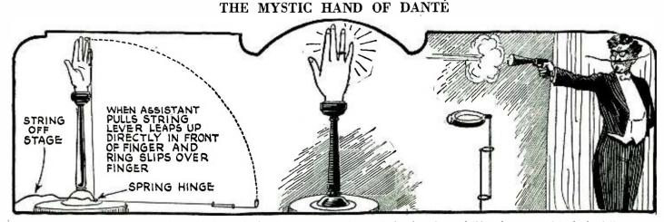
A glass hand of the feminine type is exhibited, examined and returned. It is placed in an upright position on a stand made to receive it. A lady's finger-ring is then loaded into the magician's ever ready pistol and the shot fired directly at the artificial hand where the ring appears. The magician removes the hand and presents it to the lady, who takes her ring from the glass finger. The effect is produced by affixing the
