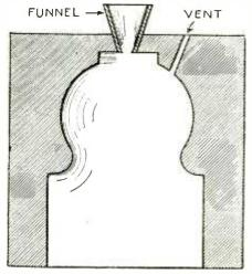
THIS IS ONE HALF OF THE MOLD READY FOR CASTING ANY NUMBER OF VASES DESIRED.
