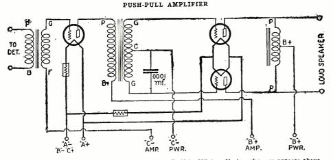
The circuit diagram for a push-pull amplifier using Radiola III-A audio transformers appears above. A small unbalancing condenser having a capacity of about .0001 mf. is connected across one-half of the secondary of the push-pull input transformer.
