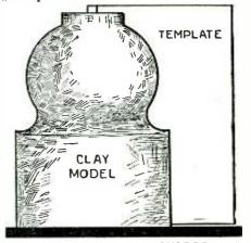
THE CLAY MODEL IS SHAPED WITH A TEMPLATE After the clay model has been made roughly, it should be shaped with a template as shown.
