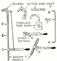
A home-made lever twig cutter can be constructed from the parts shown above. The handle is made from an old broom handle. A lever and collar (E) slip over the handle.—Tom Shivey.
