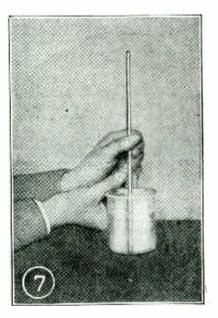
This shows a good way of increasing the delicacy of the test for magnesium. The double phosphate is precipitated better if the sides of the beaker are rubbed with a glass rod.
