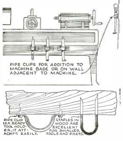
ORDINARY light sheet iron pipe clips O REFERENCE to the wall behind the machine or on the machine stand, provide perfect hangers for all kinds of tools. The clips are obtainable in various sizes. Ordinary wire staples will provide excellent hangers for small tools such as reamers, taps and drills. -G. L.
