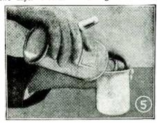
The first step in testing for aluminum and phosphoric acid is to evaporate to dryness, and dissolve in dilute nitric acid.
