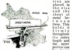
ĥe bent over and pounded down with a wooden mallet. Large sheet of metal may be bent perfectly straight when using this kink .-- Harold Jackson.
