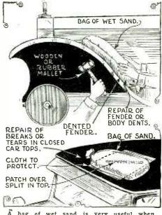
A bag of wet sand is very useful when straightening a dented fender or a body dent. A bag of sand is also of service when repair-ing a tear in the car top.
