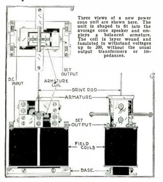
The unit shown above, a product of a New York City manu-facturer, employs a powerful electro-magnet, instead of a permanent magnet. The electro-magnet draws .3 ampere, the current being supplied from a 6-volt source.
