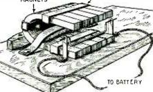
The illustration shows what may fairly claim to be the simplest electric motor. The re-quisite changes of polarity in the bent wire armature and brought about by its motions in the over-sized openings in the two standards.
