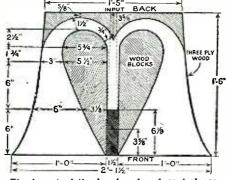
The layout of the baseboard and central sec-tion of the folded horn shown at the top is given here. The horn has a mouth area of 4 square feet and is similar to the 5-foot straight horn.
