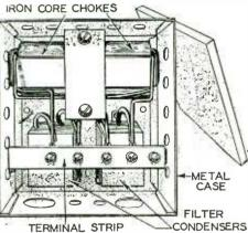
A front view of the radio interefernce filter with the cover removed is shown above. The device is housed in a ventilated metal case. furnished with the de-
