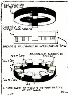
$\mathbf{T}$  HE collar shown above can be made cheaply and quickly, and will do away with the use of thin shims. The collar can HE collar shown above can be made be made in size to be adjustable to any fractional part of an inch and for use with any piece of machinery. It consists of two parts. One part is made with two keys and the other with key seats of varying depth.—G, A. Luers.
