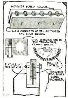
The above drawing shows a jig for holding headless set screws for machining. A block is tapped out for holding six or eight screws.
