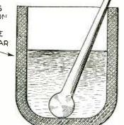
A STONE MORTAR IS USED TO GRIND THE MAGNESITE MIXTURE INTO PROPER FORM
