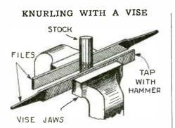
A SIMPLE and efficient means of knurl-ing can be accomplished as shown above. The work or stock is clamped beabove. tween two milling files, a moderate pressure is applied and the end of one of the files is tapped carefully, so that the work rolls be-tween the two files. Both files must be parallel and the work must be placed at right angles to them. The tangs of the files are placed at opposite ends.—*H. Pelder*.
