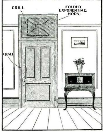
The above illustration shows how an exponential horn of the folded type may be concealed in the upper portion of a closet. The grill work covering the front does not effect reproduction in any way.
