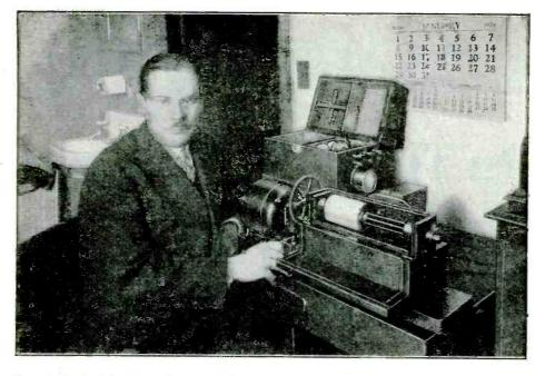
Above is Dr. E. F. W. Alexanderson and his home radio-picture receiver. Against the wall is a box containing the rectifying and amplifying units. The cover of the receiver has been lifted, showing the photographic paper.
