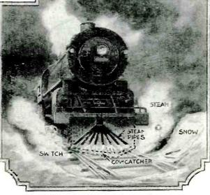
Above-A locomotive equipped with the new snow remover.
