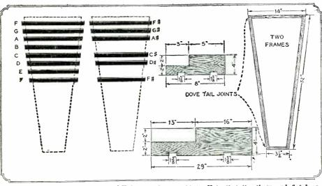
The above diagram shows how the Xylophone is assembled. Note that the sharp and flat bars are strung in groups of twos and threes and are raised on the frame slightly above the naturals. This makes for ease in handling the notes.
