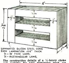
The construction details of a <sup>1</sup>/<sub>4</sub>-henry choke coil suitable for "A" eliminator work are given in the above illustration.
