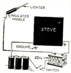
An electric match for the gas stove can be easily made from an old spark coil, a storage battery, or several dry cells, a switch and an insulated handle, as shown in the above illustration.--Glen F. Stillwell.
