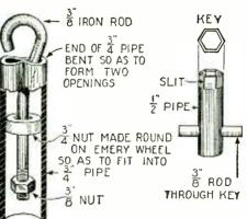
The above illustration shows the constructional details of a simple home-made lock which can be made from a few odd parts. The main portion is made from a piece of  $\frac{3}{4}$ -inch pipe, one end of which is crimped together, so as to leave two openings.—Paul Louque, Jr.
