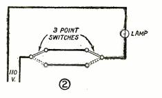
Two three-point switches connected as shown above can be used for turning a light on and off from two different locations. For two points of control, such as stairway con-trol, three-point switches are commonly used as shown above in Fig. 2.
