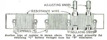
may be locked in place by turning the adjusting knobs, the shaft of the adjusting knob making contact with the resistance wire on the top edge of the strip. The sliders are equipped with insulated adjusting knobs, which simply have to be loosened and the slider shifted, in order to obtain any desired voltage.
