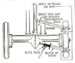
AUTOMOBILE wheels which have be-come stuck and cannot be removed can be loosened as shown above. A board is wedged for the proper tension and a jack and another block of wood are placed as shown. The wooden boards are applied to the felloe or rim.—*Contributor, send name* and address.
