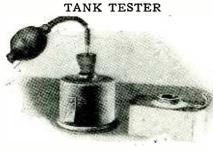
An efficient tester for small tanks and the like can be made as shown. The tank is submerged in water, and the rubber bulb pressed. Any leak will then instantly ap-pear as tiny bubbles will be noticeable. This method is better than simply submerging the tank in water, as it tests the tops also.— Wm. J. Douglass.
