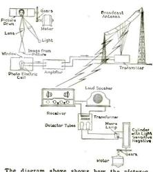
The diagram above shows how the pictures are sent and received by radio. A slotted disc, not shown in this diagram, revolves in front of the window which admits light to the photo-electric cell.
