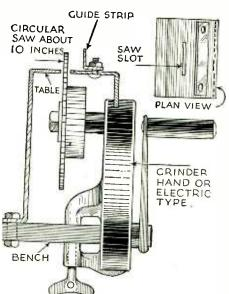
A small circular saw can be attached to the bench grinder as shown above. A saw about 10" or so will facilitate light sawing. Details of a sheet metal table top are also shown.
