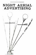
No. 1,652,996, issued to Luis Azar-raga. The object of this machine is to provide a sign which can be held aloft by a captive balloon, and further be continuously illuminated at night. The balloon is free to swing in any direction and is fastened to a tether line.
