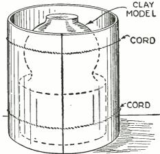
THE PLASTER IS POURED INTO · A MOLD MADE OF SHEET METAL OR LINOLEUM.
