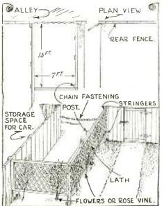
To avoid delay pending the construction of a permanent fireproof garage, a temporary shel-ter can be constructed as shown in the above illustration. A lattice work is erected, and flowers or vines are planted near it. The lat-tice work covered by flowers adds to the at-tractiveness of the rear yard.
