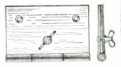
A novel method of making a small vise has recently come to our notice in the German magazine, "Technik Fur Jedermann." We are reproducing the illustration herewith for the benefit of the home mechanic. As may be seen, the device has been made from a hinge, preferably one which has mounting holes. A thumbscrew is passed through the center hole and thus the pressure upon the article in the vise may be regulated. vise may be regulated.
