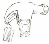
A very practical improvement to a hammer is a small claw filed in one of the two sides of the nail claw as shown above. With this it is possible to start nails which have been driven close.—F. B. Lindsay.
