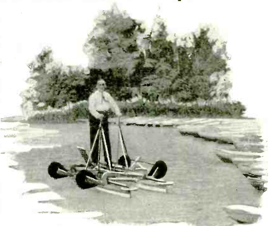
Above the "Row-cycle," as it appears in the operating position. The steering is controlled by means of pedals, and the seat slides in a fashion exactly like that of a racing boat. At left, the method of propulsion is seen to consist of a series of belts connected so as to transmit a continuous forward motion through a chain to the rear wheel.
