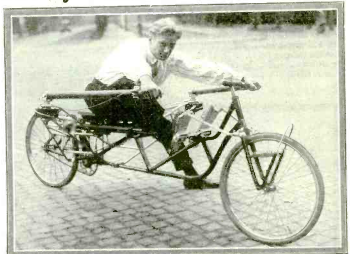
Above the "Row-cycle," as it appears in the operating position. The steering is controlled by means of pedals, and the seat slides in a fashion exactly like that of a racing boat. At left, the method of propulsion is seen to consist of a series of belts connected so as to transmit a continuous forward motion through a chain to the rear wheel.
