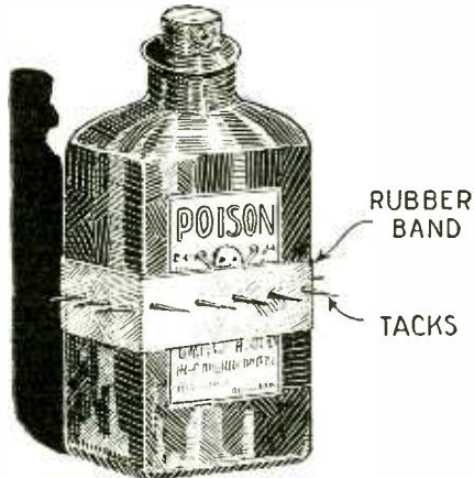
A rubber band \frac{1}{4} to \frac{1}{2} inch wide has a number of carpet tacks shoved through it from the inner side. The tacks are spaced about \frac{1}{2} inch apart and afford an excellent protection, by serving for warning as to the contents of the bottle.
