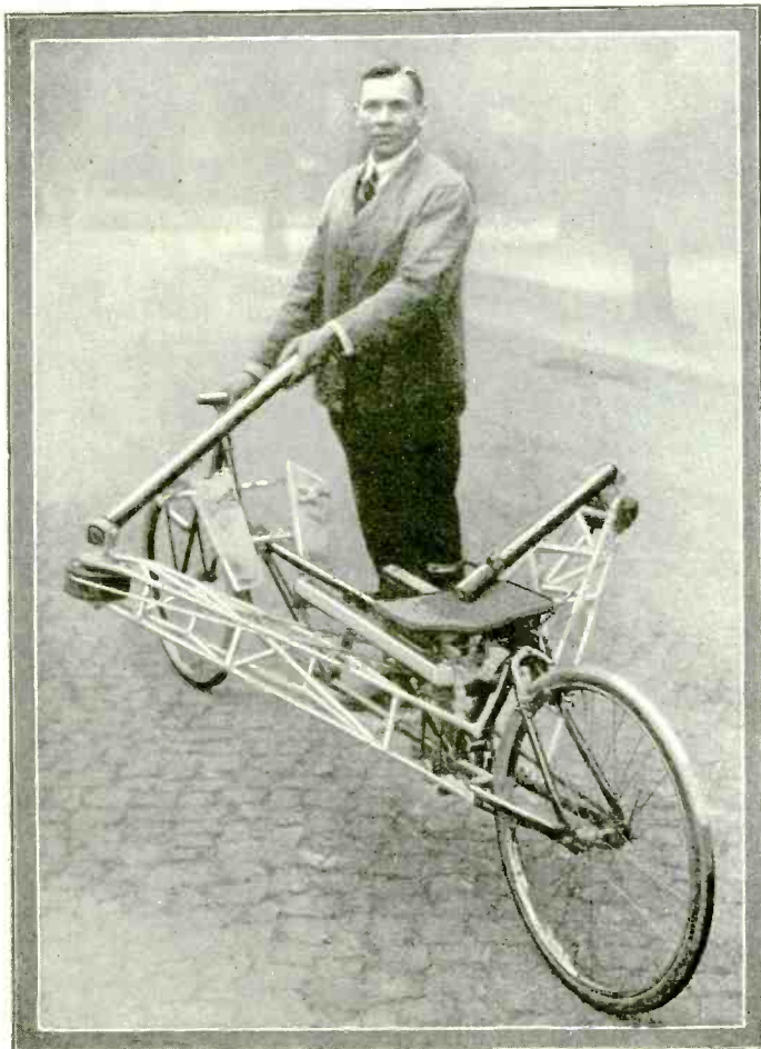
Above the "Row-cycle," as it appears in the operating position. The steering is controlled by means of pedals, and the seat slides in a fashion exactly like that of a racing boat. At left, the method of propulsion is seen to consist of a series of belts connected so as to transmit a continuous forward motion through a chain to the rear wheel.
