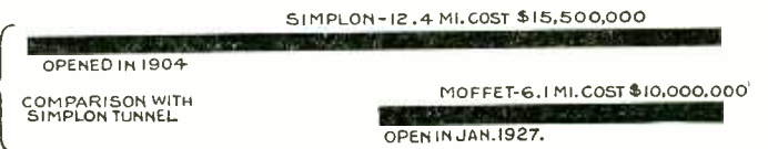
The two graph lines above illustrate comparison between the length and cost of the Moffatt Tunnel and the famous Simplon Tunnel in Europe.
