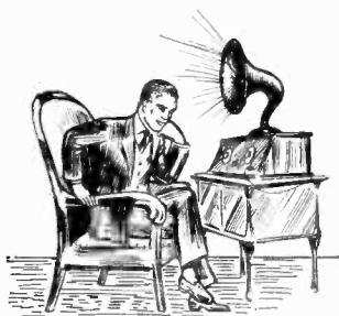
Here is shown the average type of loud speaker horn with the "morning-glory" shape. It is not the best type.
