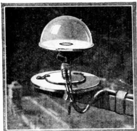
LIGHT INTENSITY RECORDER. A new pyrliometer used for studying the effect of sunlight on electrical current consumption is illustrated in the photo below. Under the glass case is a thermopile, consisting of 50 thermo-couples electrically fused together.
