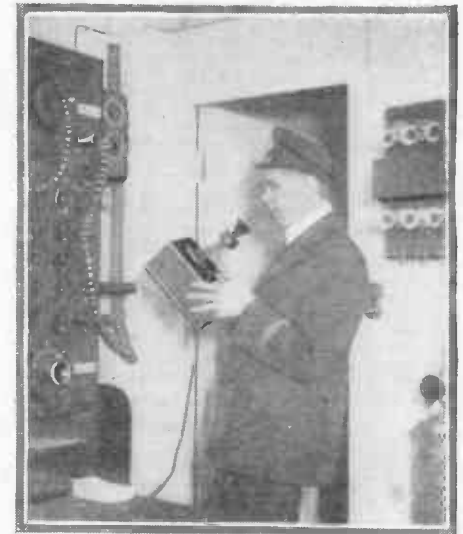
The Chief Radio Officer of the Berlin in the radio room showing part of the radiophone apparatus used for intercommunication between ships.
