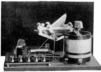
Fig. 1. A rear view of the simply designed single tube Interflex receiver, showing fixed crystal detector at right of tube socket.
