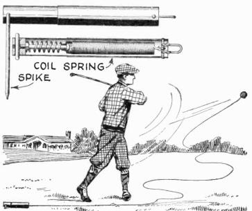
No. 1,541,420 issued to G. H. Lambert protects a device that enables golf practice to be carried on in a limited space. Furthermore, it enables the golfer to practice driving without having to chase the ball. As shown, a heavy coil spring is connected to a long cord, to the other end of which the ball is fastened. The ball is placed on a tee in the usual way and driven. It can only go as far as the cord will allow it to travel.
