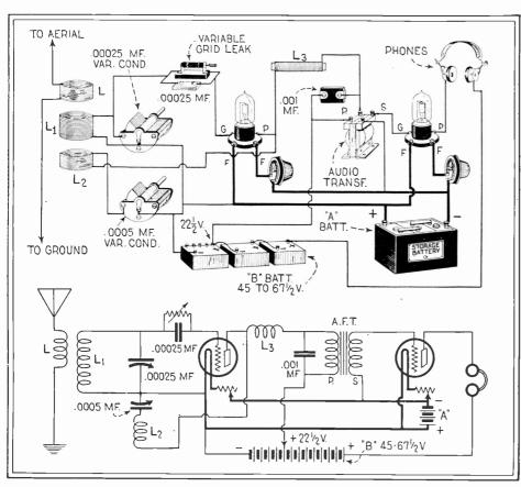
A short-wave receiver opens new fields for the radio enthusiast. An excellent type for use with headphones is shown above. The data for coils covering the 40 and 80 meter amateur band is given in the text. Follow it carefully in order to obtain the best of results.
