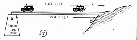
Assuming two cars on a bridge as above, with the various known factors indicated, will the pier A give way, providing both cars keep the same distance apart as indicated, and how far will the rear car be from the end B when the bridge gives way? In other words, solve the problem for the distance X when pier collapses.
