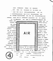
A cylindrical can, opened at one end is light enough so that it will tend to float as above. Can the can be pushed to a sufficient depth so that it will not rise when released?
