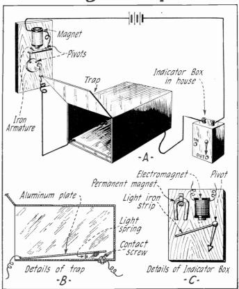
A pigeon trap that will not only catch and hold the bird but will also announce that a capture has been made is illustrated above. A bird entering the trap closes the contacts which sends the current through the indicator box and through the electro-magnet release. The door, which is heavy enough to hold itself closed, then falls and at the same time the indicator, detailed at C, shows that the trap has been sprung. Upon resetting the trap, reset the indicator by hand. —John Kautzner.
