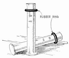
If a rubber ring such as used on suction flasks is placed around a graduate as shown above, it will prevent breakage. If the graduate falls on its side, the rubber ring absorbs the shock.
