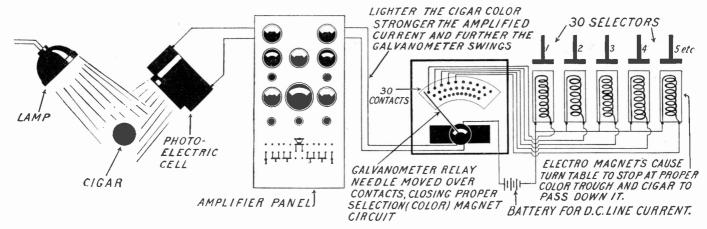
The three photographs at the top of this page show views of the automatic cigar sorting machinery which depends upon the action of a photo-electric cell for its operation. The diagram shows, in simplified form, the various instruments that make this form of sorting machine possible. Light is reflected from the cigar and acts upon the photo-electric cell to a greater
