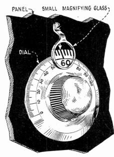
On small dials it is often hard to read the exact setting. This trouble can be eliminated by arranging a small magnifying glass directly Close tunover the pointer as shown above. ing is also simplified in this manner.
