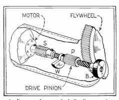
A diagram of a standard Bendix gear for automobile starting motors is shown above and described in this column.
