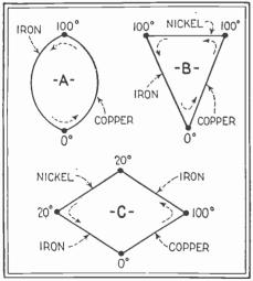
Thermocouples operate just as well with a third metal in the circuit, providing the terminals of that metal are at equal temperatures. More details on the three figures shown above will be found in the text.
