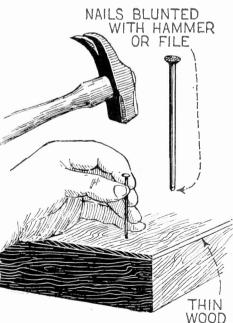
Tc avoid splitting thin wood, hammer or file the ends of the nails to a wedge shape and drive the nails so that the wedge-shaped point crosses the fibers. Much splitting of thin wood will thus be eliminated.—Max Rusch-
