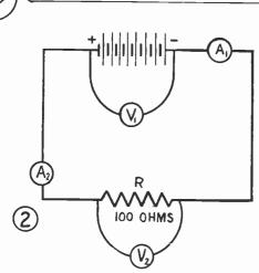
In the circuit shown in Fig. 2 above, two volt meters and two ammeters are connected in a circuit with a battery and resistance. In this particular case, which ammeter, if either, will read higher, and which volt meter?
