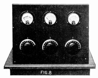
The panel containing the wave-length controls and the various meters is shown directly above. The dial indicators are scratched in the panel and then filled in with white paint.
