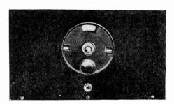
Fig. 3. The panel view of this receiver shows the extreme simplicity of tuning. Only a single tuning control is employed.
