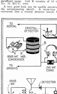
simple crystal detector circuit using the absorption method of tuning is shown above.
