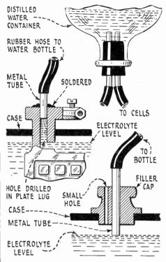
The electrolyte in a storage battery can be kept at constant level if an inverted distilled water container is placed at a point higher than the battery and is equipped with tubes, one running to each cell of the battery. Two methods of allowing the water to enter the battery are shown. All tubes must be air--I. Bront.
