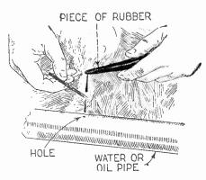
A small hole in a water or oil pipe of an automobile can be temporarily mended by melting a piece of rubber over it and allowing the drops to fall over the hole. Make a permanent repair as soon as possible as the rubber will not last. —Donald Bowie, Jr., Rep. No. 22261.
