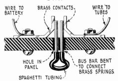
simple "A" battery switch is made from two brass contacts and a length of bus bar bent as shown.
