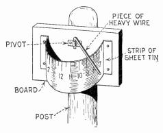
The details of a unique sun clock are shown above. To read the time, the wire arm is swung until its shadow assumes a vertical posi-The correct time is indicated by the shadow as at only one point on the dial will the shadow be vertical at a given time. The figures are inscribed on the dial by setting the sun clock each hour by a watch. In this way the clock is made quite accurate.
