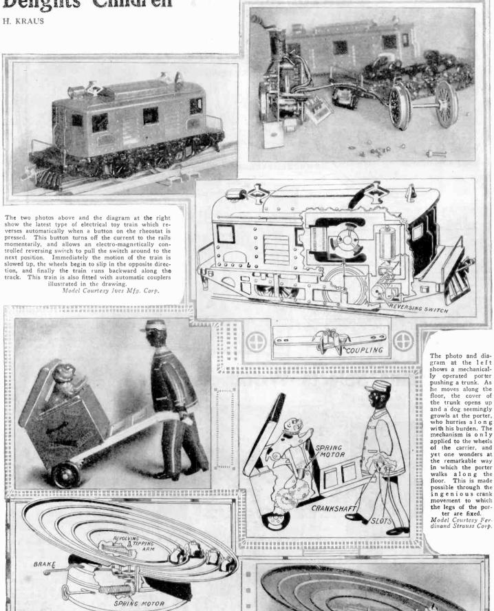
The turntable of the automobile race track illustrated above and to the right is caused to tip progressively by a small revolving tipping arm located immediately below the turn table. Four tiny automobiles are placed on the track and are caused to race around at a surprising speed. At times the innermost car will be in the lead, and at other times any of the other cars will take the lead.
