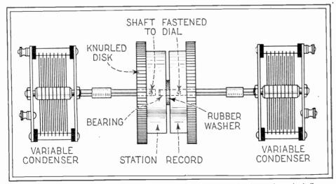
Here is a suggestion to the radio constructor that will enable him to make up a tuning unit similar to that used in this new Super-Heterodyne receiver. Variations of this method will suggest themselves. The condensers are mounted with the plates at right angles to the panel and the shafts are connected to the two dials protruding through the panel.
