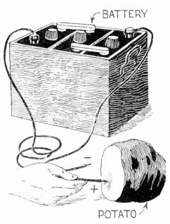
Often when a storage battery is to be used in some circuit, where polarity is an important factor in the final results, a satisfactory type of polarity indicator is not at hand and the marks on the battery are so indistinct as to be undecipherable. In such an event, cut a potato in half as above and thrust two wires that are connected to the battery into the potato. The positive wire will turn the potato green.—F. J. Wilhelm.
