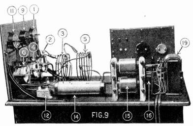
Another side view of the transmitter is shown here. The filter choke coil and the plate transformer can be seen at the right-hand end of the photograph. The R.F. choke coil is in the center indicated by 14.
