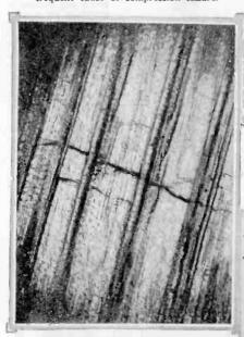
An enlarged view of a compression failure that was found in timber. This injury to the fibres was practically invisible to the naked eye but the microscope showed the fibres to be actually severed. This is shown in the enlargement above by the dark lines across the photograph.
