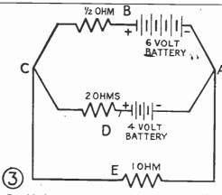
Considering the resistance of the battery and the connecting wire as negligible, which way will current flow through the branch of the circuit ADC? What effect could a change in resistance in ADC have upon the flow of current in this branch?
