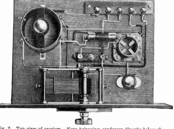
Fig. 2. Top view of receiver. Note balancing condenser directly below the fixed carborundum crystal detector of the cartridge type.
