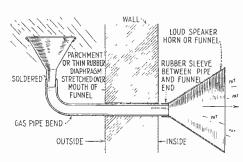
A rain alarm that requires no batteries or moving parts is detailed above. Two funnels, a diaphragm and a bent gas pipe are all that are required. The rain falling on the diaphragm produces sounds that are plainly audible at quite a distance from the reproducing funnel.
