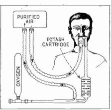
This simplified diagram shows the action that takes place in the breathing apparatus of the under-water rescue suit. See text for full explanation.
