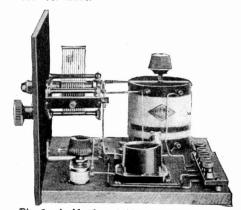
Fig. 5. A side view of this set shows the position of the filament rheostat placed directly in front of the tube socket and fastened to the baseboard. Special coupler is shown in this set.
