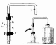
When handling liquids having fumes, the above device is useful. Attach D to a suction pump. A partial vacuum is created Attach D to the bottle being filled and the liquid from the large bottle passes into the small one through the long bent tube.
