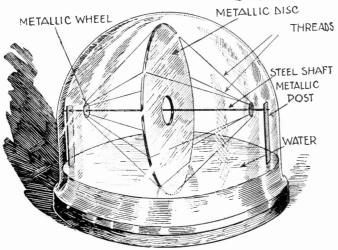
An interesting motor that will revolve without any visible external source of power is illustrated above. Two different types are shown. The uppermost can be quickly and easily made from a spool, several lengths of thread and a suitable wire axle. Assembled as shown, the wheel will turn about one revolution every 8 minutes. A more elaborate model may be made as shown in the lower part of the above illustration.
