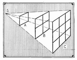
A diagram showing graphically how the intensity of light varies inversely as the square of the distance. S. A. B and C are equal distances apart.
