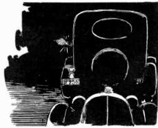
No. 1,548,916 issued to J. R. Thompson describes a night signal device for automobiles that requires no mechanical or electrical connections and that always operates if the lights of following cars are turned on. It merely consists of a red reflector strapped to the wrist of the driver. All of the standard hand signals can be given with this device in use.
