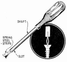
screw driver that will hold a screw while it is being started in an accessible place is made by using two spring steel strips as above. -J. E. Tewksburg
