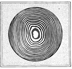
Newton's rings formed as described here take the appearance illustrated above. Note the gradations of widths of the rings.
