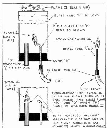
We know that a gas flame burns in air but will an air flame also burn in gas? This experiment answers the question. The apparatus necessary is shown. Connect the glass tube to the gas supply. Open the gas valve slightly and light. As long as the flame is small it will burn but if turned on full, the flame will die out. At the same moment an air flame will form automatically on tube D and we can light another gas flame II at the top of the large glass tube.
