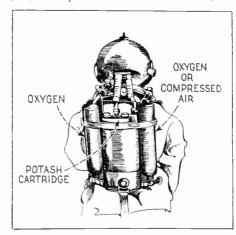
Rear view of an up-to-date diving suit showing oxygen tanks and potash cartridge for regenerating the air supply.
