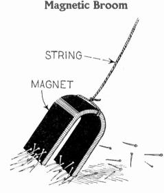
When a quantity of nails or other small iron or steel objects are spilled on the floor, they can easily be picked up by means of a magnet suspended on a string as shown above. The magnet is drawn across the floor several times and when picked up will be found to bring all of the magnetic objects with it. In this way, a job that was formerly tedious can be performed with little effort and in a small fraction. Go the former time.—E. L. Dunbar,
