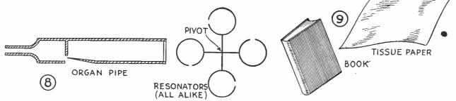
If four resonators are mounted on a pivot so that they are perfectly free to rotate and if they are all alike, which way will they tend to rotate when a blast is blown on an organ pipe to which they are tuned?
