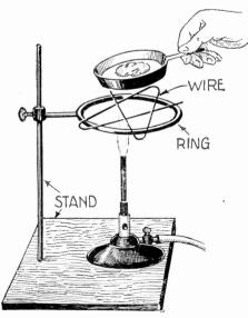
In the chemical laboratory, often large ring stands only are available. To support small evaporating dishes or other apparatus on them, bend a piece of wire into the shape shown above and support the receptacle thereon. In some cases, two large wire hairpins can be laid across the ring, with the same results. This kink is one worth bearing in mind as it will often come in handy.—
