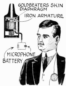
No. 1,545,525 issued to H. Sell protects a novel type of very small telephone receiver that fits into the ear and requires no head band or other holding device. The details of one of the receivers are shown in the upper left-hand corner and the device is illustrated in use above. It can be used for various purposes, the most important being as an aid to people hard of hearing.
