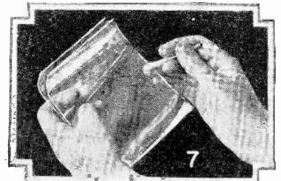
↑ The photo above illustrates how two old films are cemented together for making the card case illustrated in photo 8.
