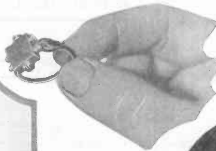
A complete radio receiver built in a finger ring. The detector and capacity and inductance are enclosed. Four binding posts provide connection to aerial, ground and phones. —Carl G. Peterson.
