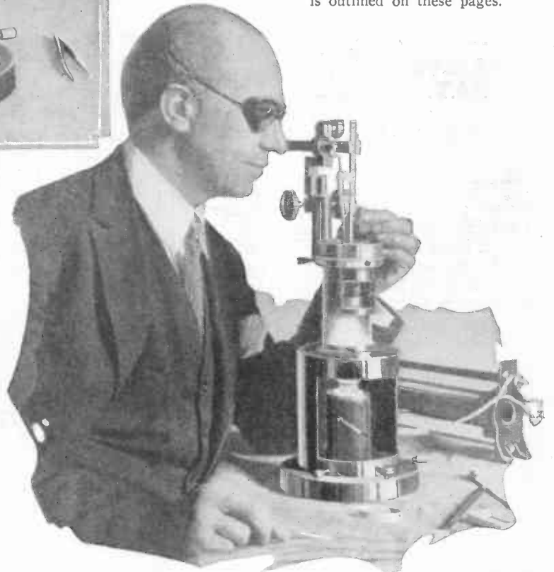
Above: Operating the modified Rosenthal lucidoscope used in detecting the genuineness of pearls.
