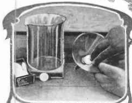
Above: Preparing the filter to be used in the process of purifying shellac. Either ordinary folded filter paper or the type shown may be used.
