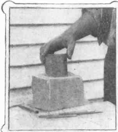
Above: When a cavity is to be in the finished object, it is formed in the still plastic clay with a round tin can.
