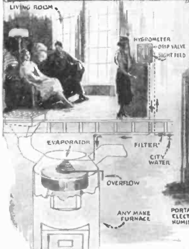
A decorative casing to be placed around radiators and to contain water for humidifying the air has recently been placed on the market. It is illustrated in perspective and cross-section.
