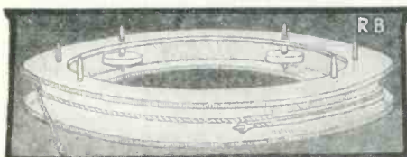
This picture shows detail and close-up view of the roller bearing collar "RB," in which are placed six friction wheels as shown, these serving to spin the dancing girls as they circle the temple.
