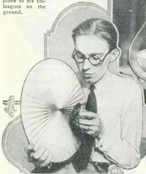
A cone type loud speaker made of pleated paper is one of the latest types of reproducers guaranteed to reproduce all overtones without causing distortion, or in any other way altering the true rhythmic qualities of the music.
