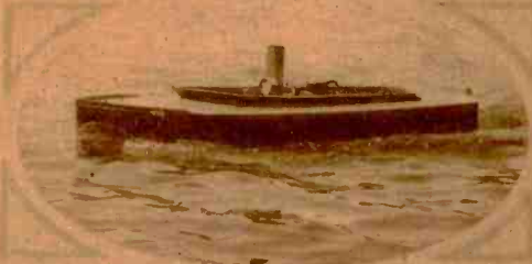
Above: A model of a steam power boat is shown traveling at full speed. This model measures 48" over-all and is capable of a speed of 12 miles per hour. The boiler is tested to 200 pounds pressure.
