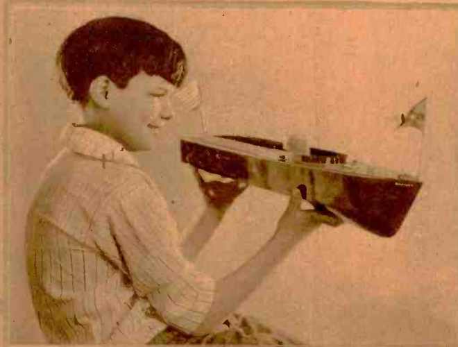
The vessel shown above can be obtained in knock-down form or complete. It is steam-driven, and has a four-cylinder engine and a steam boiler which supplies a super-heated steam to the driving mechanism.
