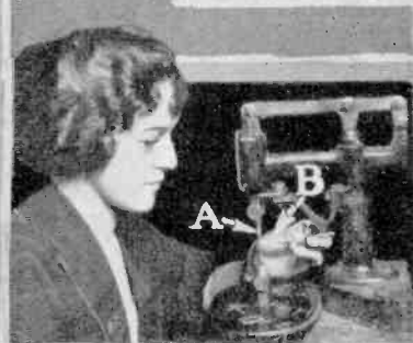
The above illustration shows a small foot-fed arc, the electrodes indicated by A. This arc is used to weld the filaments into vacuum tubes. The elements are indicated by B. It is impossible to use solder in this place.
