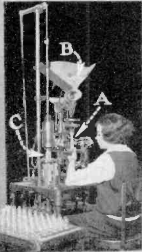
Above: The machine which performs two operations on the glass bulb. At C, a hot flame is directed on the top and a hole blown therein. At A, a glass tube from hopper B is sealed to the opening thus formed. This tube is to be used in a later step for evacuation.
