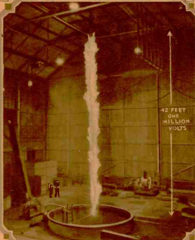
A forty-two foot controlled arc! It hardly seems necessary to add that this is the longest controlled arc ever made. One million volts transmitted to the ends of the conductors between which the arc occurred was necessary to produce this arc. It was drawn in tests for "Wet Flashover," which is a test applied to the conditions under which high tension lines must operate in rainy weather. Accurate comparison of the hugeness of this discharge may be gained by comparing the thickness of the flash as well as its length with the size of two men shown standing in the photograph. The arc was held under perfect control.
