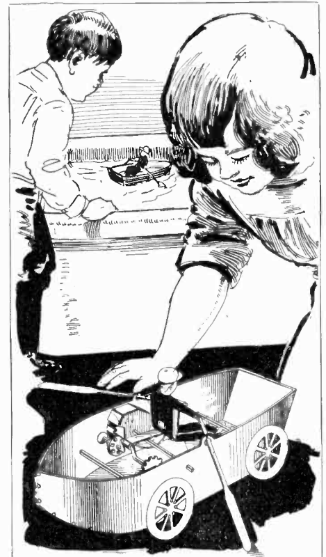
(Pat. No. 1,456,429, granted to Joseph L. Duggan.) The body of this toy is made of light metal. It is fitted with wheels, although it is built in the form of a boat. The spring motor it contains is connected to the wheels through a chain of gears and to an upright piece fastened to the figure in the boat holding the oars. When on land the boat is driven by the wheels; when it is in water the oars move it. Both the wheels and the oars move continuously. The figure holding the oars is pivoted where it is attached to the seat in the boat. The oars are also pivoted.
