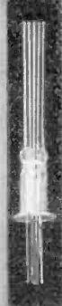
Left: The form on which the elements—the grid, plate and filament—are placed. Note that five wires extend above the glass tip while only four go below. The odd wire supports the grid.
