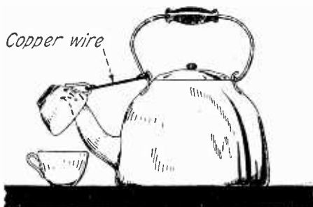
A Simple Still May Be Made By the Use of Two Cups and a Tea Kettle.
