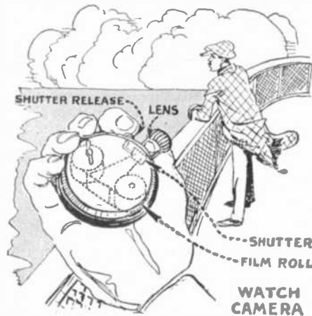
The Detective's Pocket Watch-Camera Containing Lens, Shutter and Film Magazine. The Author Describes How He Took Several Pictures in This Way of a British Ambassador on Board Ship Much to His Surprise and Amusement. He Never Knew That He was Being Photographed.
