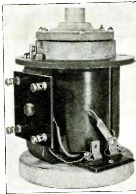
Loud-talker design, model of which was tested in Radio News Laboratories, as built by Mr. H. L. Jones, third prize winner. All details are given in the text and accompanying drawing at the right.
