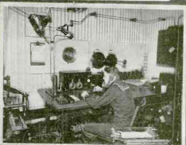
The receiving set situated in the transmitter room is shown herewith. The motor-generator are controlled by a switch on the lower left hand corner of the table. The wheel controlling the wave changing switch can be seen at the left hand side of the photo.
