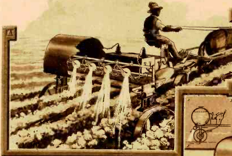
Dr. Miller Reese Hutchison, famous electrical engineer formerly with Thomas A. Edison, here proposes two schemes for annihilating the cotton weevil. The first scheme he proposes is that involving the treatment of the cotton plants with powerful X-rays, as shown above; a second scheme is to spray the plants with salt water and to pass an electric current through the spray of water, thence through the plants and earth, and back to the battery as the arrows in the insert diagram clearly show.
