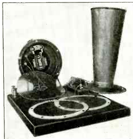
Fifth prize winner in the Loud-talker Contest. This loud-speaker is built almost entirely from a Ford automobile horn, a moving coil being fastened to the diaphragm in the manner shown.
