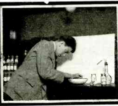
Testing soil with litmus paper, to determine whether it is acid or alkaline.
