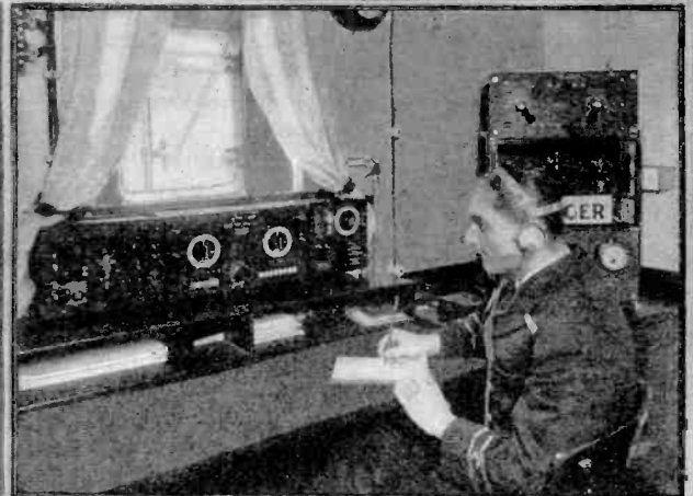
The Receiving Set in Another Part of the Radio Room is Here Shown. The Apparatus in Back of the Operator is a Three Tube Transmitter.
