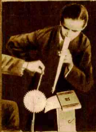
The Siren—Each Speed Gives a Different Note, Reinforced by Air Thru a Paper Horn.
