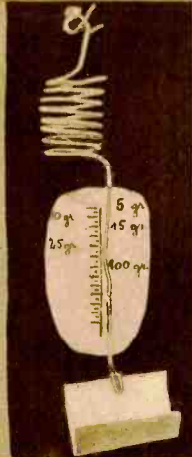
A Long Piece of Wire Is Twisted Around a Pencil, Forming a Spring; a Scale Can Be Made Thus.
