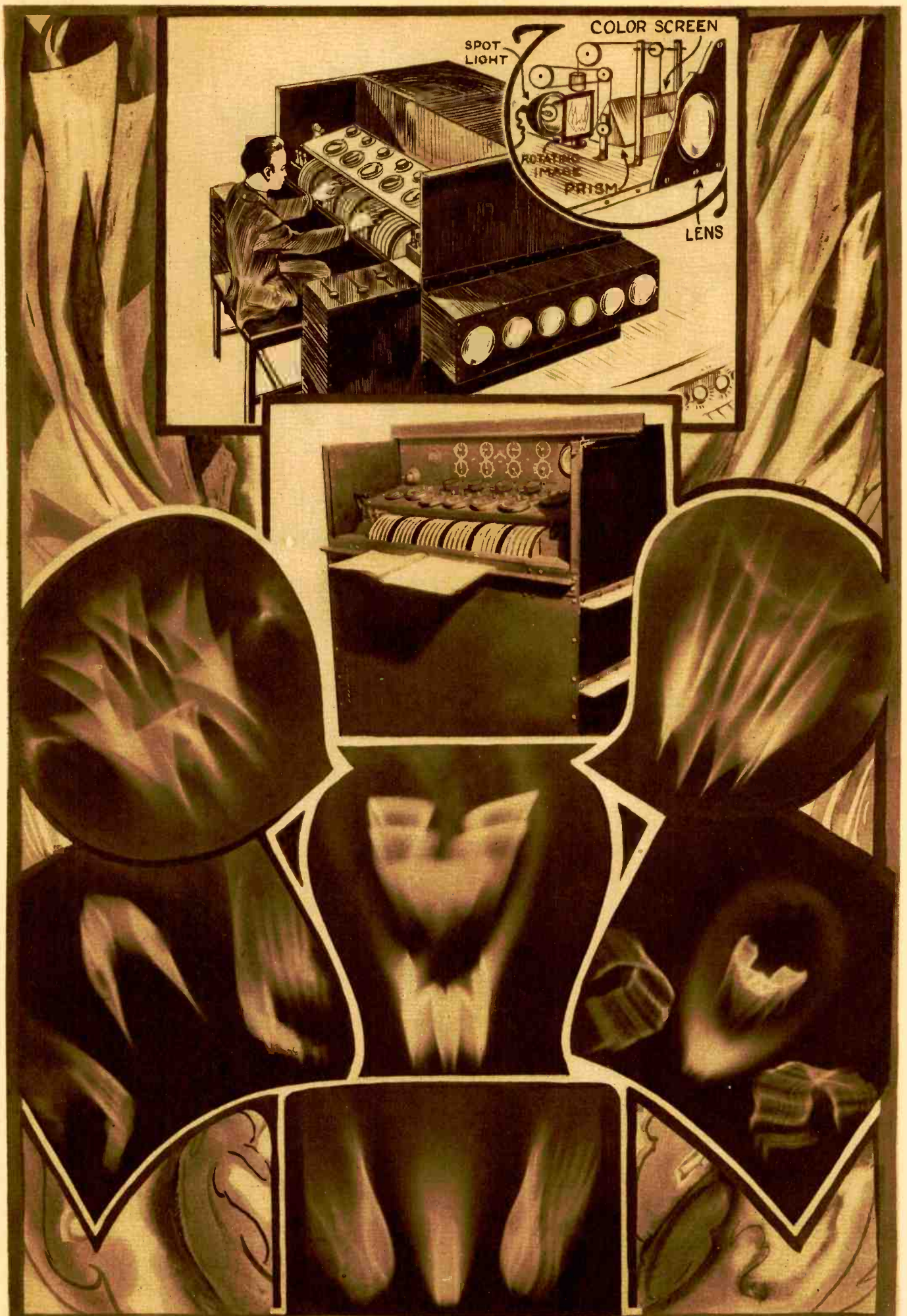
The Specially Prepared Diagram at the Top Shows How the Color Organ Produces the Marvelous Interblending Color Effects on a Ground Glass or Cloth Screen; While the Six Lower Photos Show Some of the Different Image Effects Obtained. The Center Photo Shows the Keyboard of the Color Organ.
