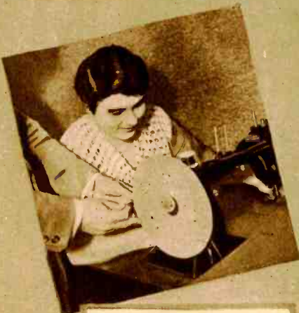
A Disk of Strong Cardboard Attached to a Sewing Machine Gives a Rotary Saw. At High Speed It Will Cut a Pencil.
