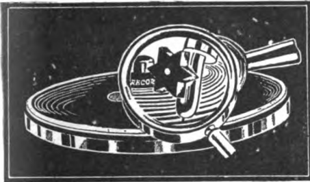
A Renewable Needle for Feeding Down a Wire Which Constitutes the Playing Stylus. Here Takes the Place of the Usual Phonograph Needle. The Amount of Its Projection Affects the Playing, Making It Loud or Soft.
