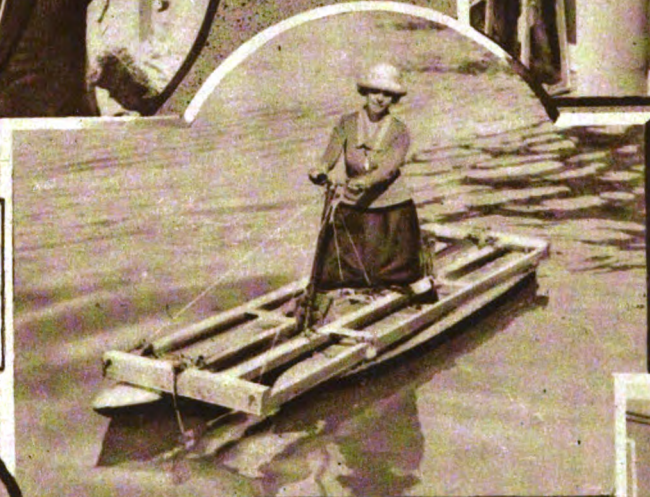
Miss Velma Tilden, of San Francisco, is Shown Attempting to Cross San Francisco Bay in Sheldon's "Water Walker." The "Walker" is Built of Sheet Metal and Consists of Two pontoons Sliding in a Frame Work. Hinged Metal Fins Fold Back and Slip Thru the Water as the Walker's Foot Pushes the Pontoon Ahead.
