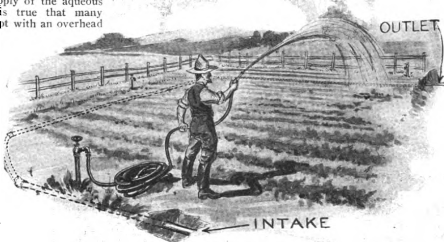
We Know That It Is Impracticable for Farmers to Water Their Crops by Running Sprinkler Pipes Over the Fields, as These Would Interfere With the Cultivation of the Ground, such as Plowing, Etc., but Says Mr. Hobson, Why Would it Not be a Good Idea to Place the Necessary Water Pipes Under Ground, and to Provide at Suitable Intervals Short Pipes and Valves Projecting Above the Ground for the Attachment of a Hose?
