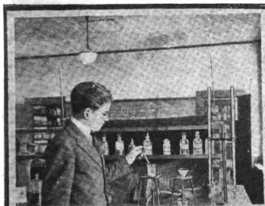
Left—Dissolving Soap Preparatory to Filtering and Titrating for the Amount of Alkali Present.
