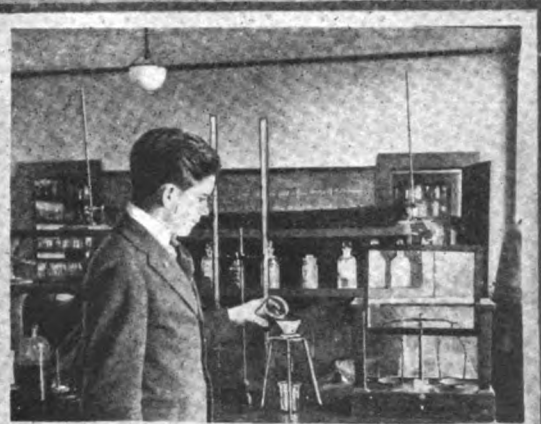
Left—Weighing Out a Sample of Tartaric Acid for Titration in Determining Its Purity.
