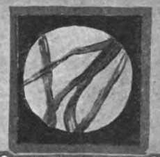
Microphoto of Paper Fibers, Compare With the Microphoto Below of Cotton Fibers.
