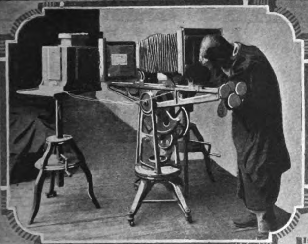
French Scientists Have Contributed a Great Deal to the Cutting Down of Crime, and Electricity as Well as Chemistry and Photography Have Been Harnessed so as to Work Hand in Hand as an Aid to the French Detective Forces. The Photo Above Shows an Expert Examining a Suspected Bank Note for Erasures by Photographing the Bank Note, by Means of Ultra Violet Light, all Other Actinic Light Being Screened Off.
