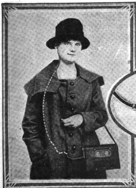
Here We Have the Latest German Invention—an Extremely Small Yet Complete Telephone Set to Aid the Deaf in Hearing Better. The Receiver Which Fits into the Ear is Smaller Than an American 5c Piece. The Microphone and Battery are Carried in the hand bag.
