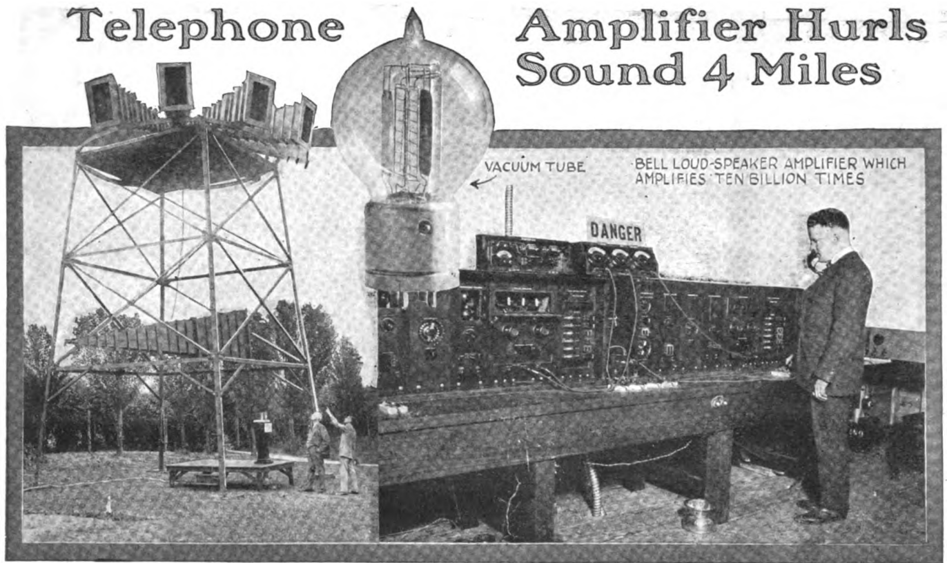
Recently Music was Transmitted Thru the Air for About Four Miles and a Spoken Voice Told Its Story About Three Miles From the Large Wooden Horns, Shown at the Left of the Illustration. The Original Voice Actuated an Ordinary Microphone, Such as We See on a Desk Telephone Set, and When This Current Was Received in the Laboratory, Shown at the Right, a Large Number of Vacuum Tube Amplifiers or Audions Boosted the Voice Ten Billion Times. The Receiving Station was Located at Napanoch, N. Y.
