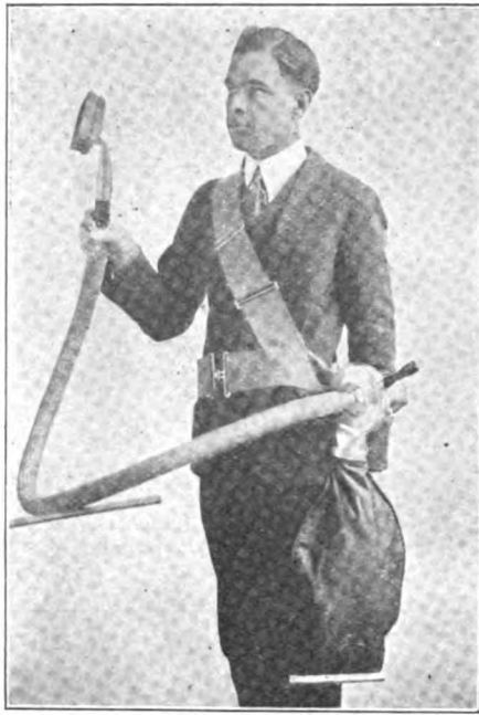
Our Cut Shows the General Service Vacuum Cleaner and Operator, Illustrating the Method of Attachment to the Person, and Showing How Conveniently it Can Be Manipulated.
