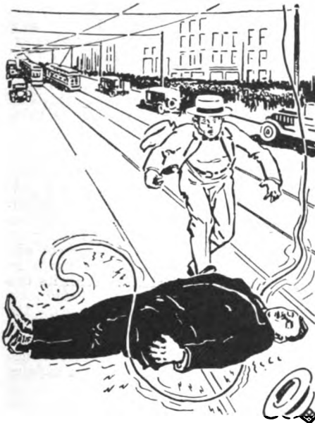
Fig. 7—Caught in Trolley Wire. Be Careful Not to Get Shocked in Rescuing Him. Heavy Rubber Gloves or a Dry Coat, Dry Wood, Sticks, Etc., May be Used, but Don't Touch the Victim's Body With the Bare Hands.
