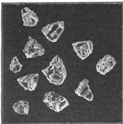
These Eleven Stones, Made in Nine Hours, All Measured Over One-Twelfth Inch in Their Greatest Diameter. They Were Produced in the Electric Furnace, With a 700-Ampere Current and at a Potential of 32 Volts.
