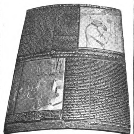
Actual Appearance of Curved Electrotype Used in Printing Page 30 of the "May" Issue of Science and Invention
