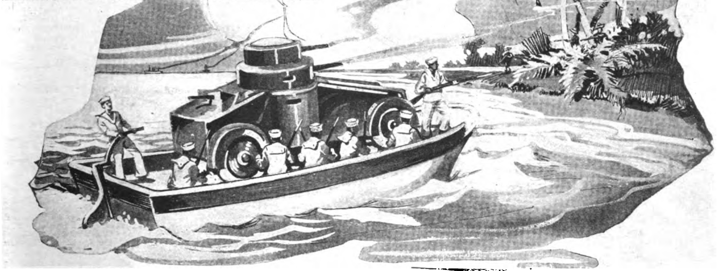
A Recently Patented Idea Which Will Find Extensive Adaptation in Future Warfare Maneuvers, Especially in Landing Troops or Marines as Here Shown. The Armored Motor-Car Is Caused to Propel the Landing Boat By Placing the Hind Wheels On a Series of Friction Rollers, Suitably Gearing to the Propeller Shaft in the Manner Indicated in the Diagram at the Top of the Illustration. The Guns of the Armored Motor-Car Can Be Used While the Boat Is Moving, When Desired. The Front Wheels of the Motor-Car Rest in Grooved Chocking Blocks.
