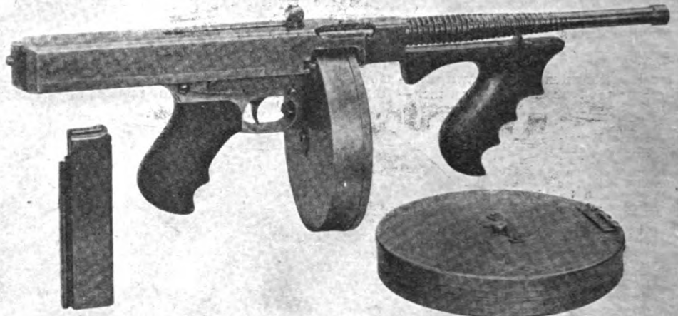
The Illustration Above Shows Close-up View of Submachine Gun With Pistol Type of Magazine at Left, and Circular Drum Magazine Holding 100 Cartridges, at the Right.
