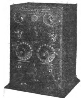
Type P-300 Combination Audion—UltraAudion and One-Step Amplifier
