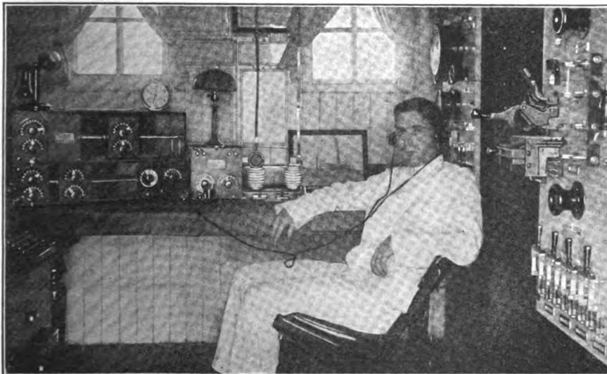
This is the Way Things Look Inside a Ship's Radio Cabin. In This Case, You See a Pioneer Operator, Mr. E. D. Frey, Waiting for an "SOS" on Board the Palatial S.S. "Abascoz." By Way of Instruments, the Famous "Double Decker" or "I.P.78" Receiving Tuner May Be Seen to the Extreme Left. No, Young Man the Desk Telephone on Top of the Tuner Does Not Connect to Shore Stations but Is for Direct and Instant Communication to the Vessel's Navigating Bridge.
