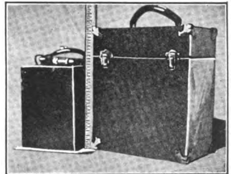
View of the Long-Wave Receiving Set with Carrying Cabinet Closed, Compared with Rule. The Cabinet Measures About 14 Inches High and is Fitted with Leather Handle and Snap Locks, Which Can Be Purchased From Any Trunk or Leather Goods Supply House.
