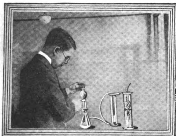
At Left: Generating Sulfur Dioxid and its Action in the Bleaching of a Rose.
