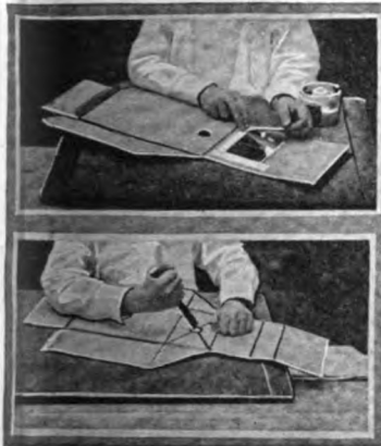
The Successive Stages to be Followed in Constructing the Home-Made Stereoscope Here Described by the Author, is Clearly Shown in the Progressive Series of Photographs. The "Modus Operandi" of the Apparatus is Shown Clearly in the Diagram at the Extreme Right. The Photograph or Picture to be Viewed Stereoscopically is Placed Under the Bottom of the Box Adjacent to the Opening Thru Which the Necessary Light for Illuminating the Picture Passes. The Eye is Placed Before the Lens Opening, as Shown, and the Reflected Image of the Picture in the Mirror Mounted at an Angle in the Top of the Case Causes the Details and Objects in the Picture to Stand Out in Relief, the Same as in the Regular Double-Lens Spectroscope Requiring Special Duplex Photographs. The Present Instrument Uses Any Photographs or Pictures You May Have. Many Pleasant Hours May Be Spent with the Use of This Simple Home-Made Apparatus, Which Costs Practically Nothing to Build.
