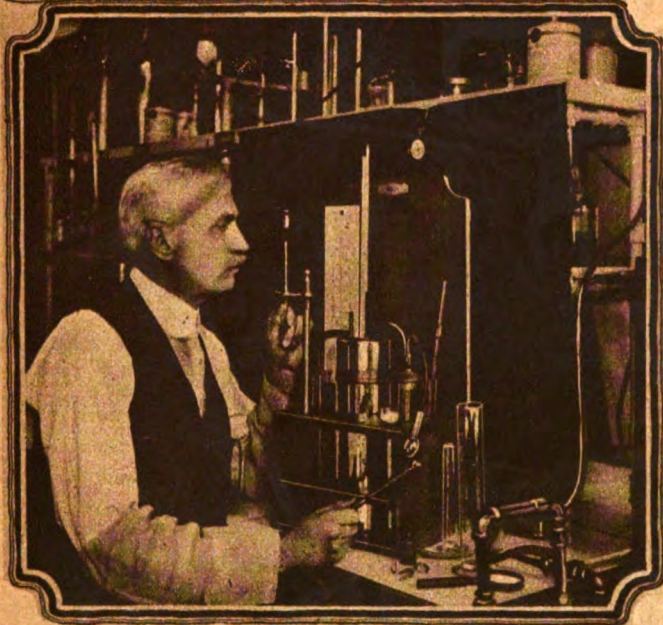
Makes Milkmen Fear Water! The "Cryoscope," which in eight minutes enables one to tell just what amount of water has been added to a sample of milk. Until the invention of this new testing apparatus, which is based on the principle of the "freezing point" test, no suitable rapid method for detecting dishonest milk dealers had been perfected.—Photo by Gilliams Service.
