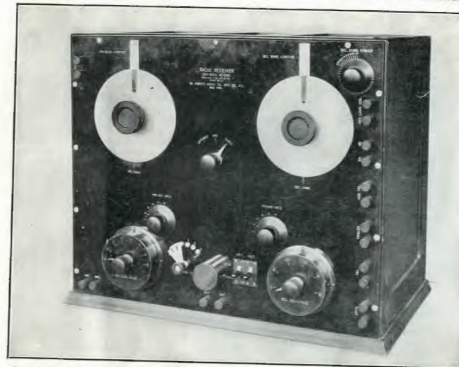
Latest De Forest Radio Receiving Set With Calibrated Inductance and Condenser Knobs Enabling The Wave Length of an Incoming Signal to Be Instantly Determined. Adapted to Damped and Undamped Waves.
