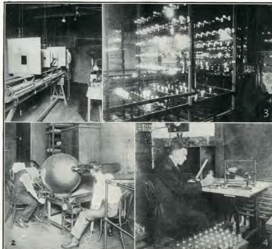
Fig. 1. Shows a Photometer for Measuring the Candle-power of Incandescent Lamps. Fig. 2 a Spherical Photometer for Similar Work. Fig. 3. "Life" Test Racks. Fig. 4. Lamp Inspector at Work.
