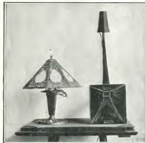
The Lamp at the Left Contains a Microphone and Loud-Talker; Improved Loud Talker with Horn at Right.
