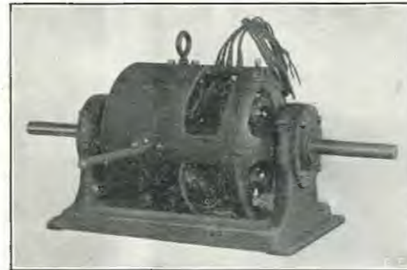
Simple Form of Dynamometer for Measuring Horse-power of Small Engines and Other Machinery.
