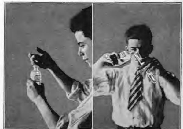
Fig. 8-A, (left), Grasp Glass Stopper of Bottle Between Third and Small Finger. Fig. 8-B, (right) Shows How to Thus Retain Stopper and Pour Out Liquid.
