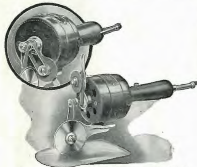
Electric Cloth Cutter and Method of Sharpening It. Latest Adjunct to Tailoring and Dressmaking.
