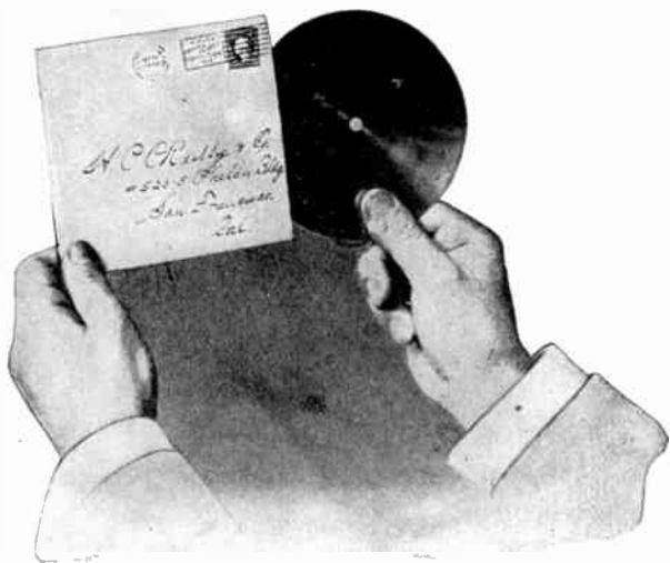
The Latest Telegraphone "Dictation" in the Form of Thin Steel Discs May be Mailed; the Recipient Transcribing the Speech Record on His Machine.
