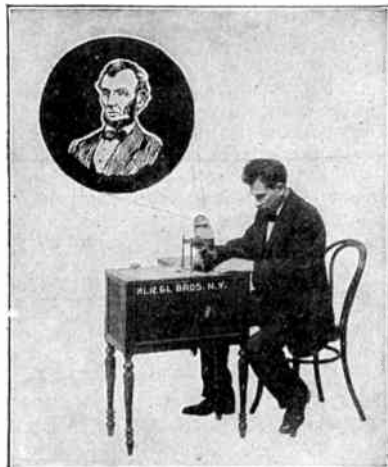
Fig. 6. A Special Projecting Lantern with Which It Becomes Possible to Show Cartoons Being Drawn by the Artist
