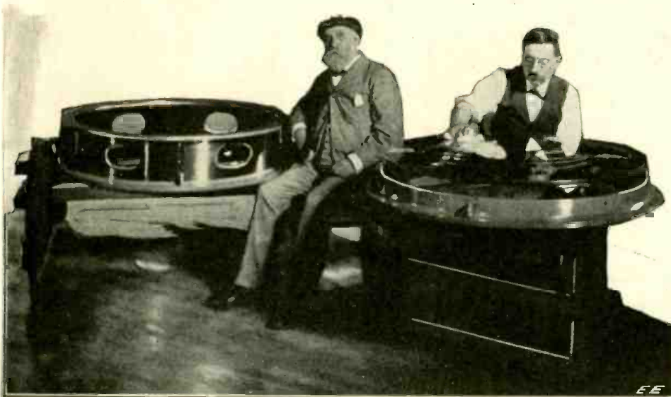
The Glory of the Glass Maker Is Undoubtedly Reflected In the Large Telescope Lens, the One Here Shown Being One of the Most Perfect of Its Kind In the World, and Measuring 40 Inches in Diameter. The Reflection of the Man's Image at the Extreme Right Will Be Noticed on Close Inspection. Frequently a Great Many Batches of Glass Have To Be Run Off Before a Sufficiently Perfect Block of Glass from Which to Grind the Lens of This Type Is Obtained.
