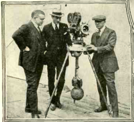
Motion Picture Camera Mounted on Gimbals Devised by C. E. Shurtleff, for Purposes of Taking Motion Pictures on Shipboard. The Contrivance Was First Tried Out in the Filming of the All-Star Production of "The Mutiny," from Jack London's Novel, "The Mutiny of the Elsinore." It Keeps the Camera Level, No Matter How Rough the Sea. C. E. Shurtleff, the Inventor, Appears at Left.
