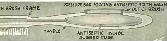
Wouldn't You Like a Tooth-brush Like This One?—Squeeze the Handle and—Presto! You Have the Mouth-wash Post-Instantly.
