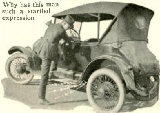
Step on This Running Board and the Klaxon Walls Out Its Warning.
