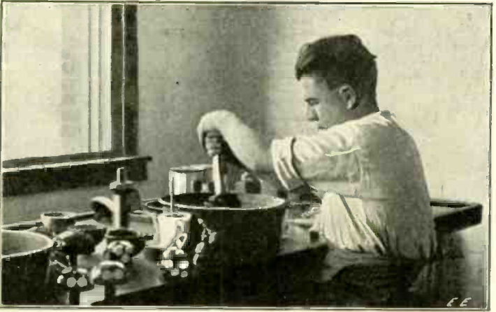
The Fine Grinding of a Camera Lens. The Lenses Are Mounted In Polishing Heads and By Means of the Handle, the "Head" is Given a Circular Motion In a Polishing Trough, With Rouge and Certain Other Fine Abrasives Used as Grinding and Cutting Agents.
