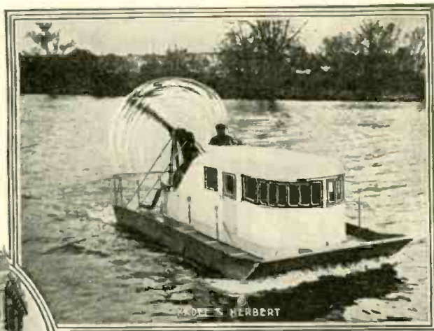
A New Type of Air-Propelled Boat Built by the French Which Makes a Speed of 74½ M.P.H. on a Half Mile Basis. This Speed Performance Probably Constitutes a World Record. Various Types of Gliders Are Now Practicing on the Seine for the Coming Monaco Races. The Photo Shows the De Lambert Glider, Which Has Been Designed for Passenger Service on Shallow Waters, Driven by an Aviation Engine.
