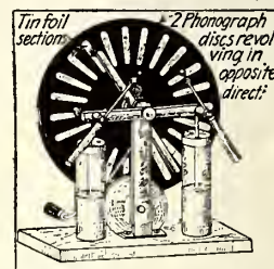
Two Old Phonograph Records Make a Good Static Machine, When Drest Up a Little With Some Tinfoil Sectors, and Then Rotated in Opposite Directions.
