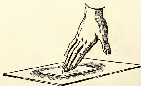
Fig. 1. The Principle of the Gliding Railway. Two Glass Plates are Dipped into Water. The Upper Plate Will Glide with Astonishing Ease. The Two Plates Do Not Touch. A Thin Water Film Separates Them.
