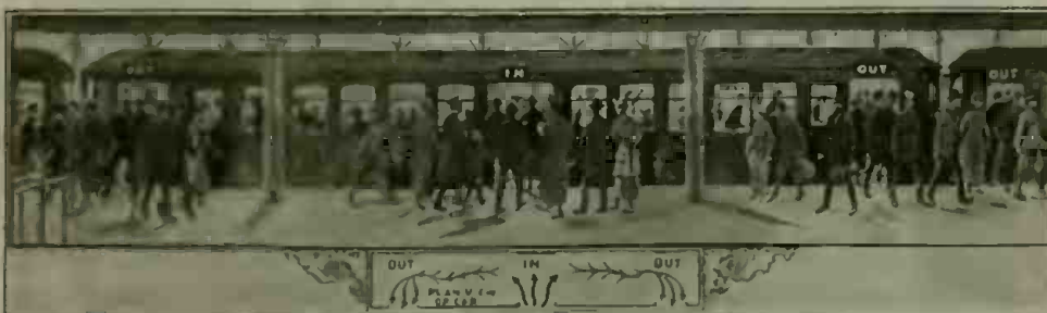
The Cure for the "Subway Crush".—There Are Three Doors on Each Subway Car: Two on Each End and One, About the Same Size as the Front and End Door Combined, in the Center. Let the Outgoing Passengers Use the End Doors Only, and the Incoming Travelers the Center Doors Only, as the Diagram Indicates.
