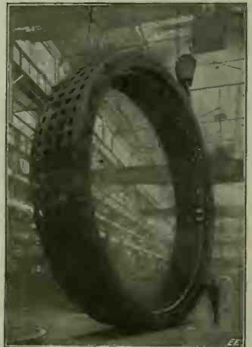
Note the Relative Size of the Man Compared to the Huge Stator of the Largest Water-Wheel Type Generator Ever Built. It Develops a Current of 11,000 Volts.
