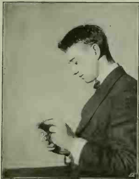
Fig. 19. The Burning Test Applied to Various Cloth Materials to Determine Their Composition, Particularly the Presence of Wool. Vegetable Fibers May Be Readily Distinguished from Animal Fibers by Burning, Animal Fibers Such as Silk and Wool Giving Off the Smell of Burnt Horn. They Do Not Fire Like Vegetable Fibers, But Cease to Burn When Removed from the Flame. Vegetable Fibers Give Off a Slight Odor of Burnt Wood When Ignited, and They Burn Away Very Rapidly With a Flash, leaving No Hard Cinder, But a White or Gray Ash Only.
