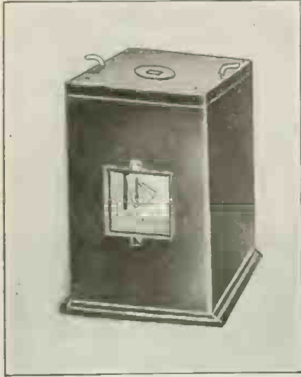
Appearance of Finished Electroscope Especially Designed for Conducting Experiments in Radio-Activity.
