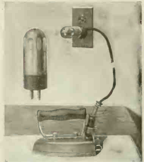
Something Every Housewife Wants—a Positive Indicator That the Electric Iron Is "On" or "Off." The Tell-tale Lamp Solves the Problem.
