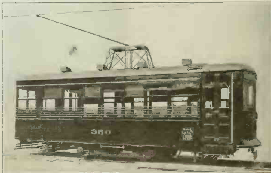
In Marked Contrast to the Early Trolley Car Shown Above, Is this "One-man Automatic Trolley." It Is Built Like a Machine Gun. The Motorman Controls the Power, Brakes, Track Sander, Door Openers, Collapsible Steps, Bell and Lights.
