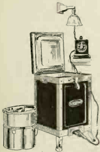
The "Fireless Cooker" Principle is Incorporated in This Electric Stove. You Start with 620 Watts for a Few Moments, Then Switch on the 40 Watt Heater, the Latter Doing the Real Cooking.
