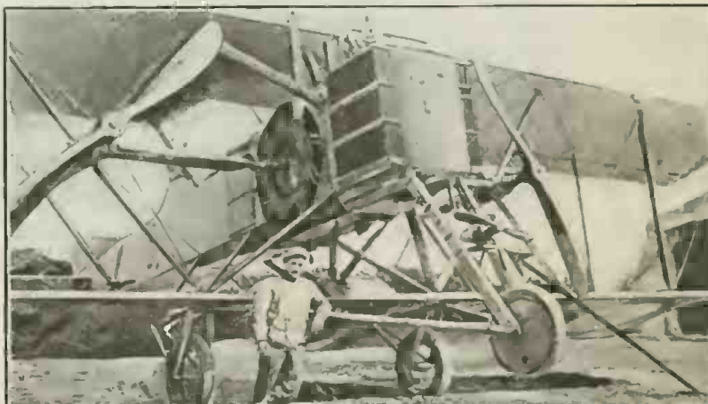
This Photograph Shows Clearly How a French Aeroplane Is Equipt with Radio. The Transmitter Is Supplied with Current From a Small Dynamo Driven By the Small Air Propeller Marked By the Arrow In Top Photo. Lower Photo Shows Transmitting Key and Instruments.
