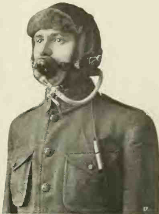
U. S. Aviators Are Being Supplied With the New Dictograph Here Shown, for Carrying on Conversation With a Second Officer, While in Flight. The Engine Noise and Wind Make It Difficult to Talk Otherwise.
