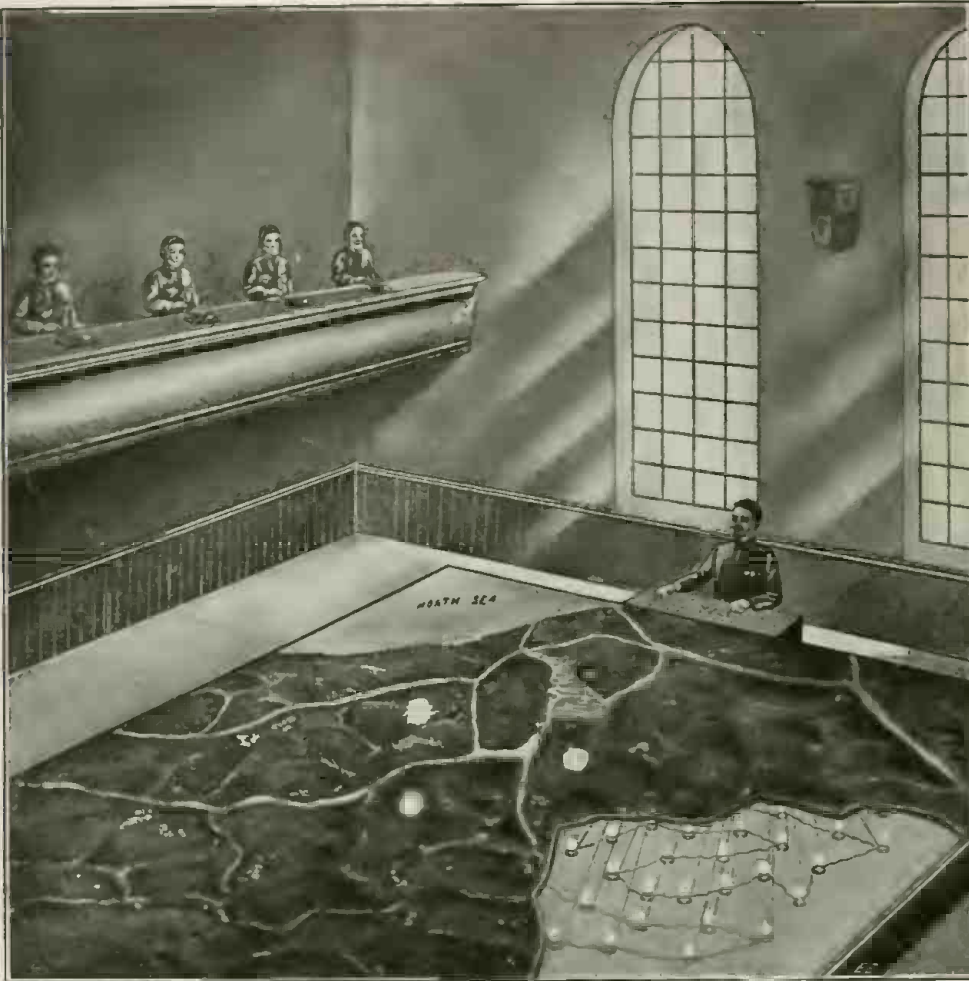
The U. S. Aviation School At a Western University Has Adopted an Electric Map for Coaching Future Birdmen. The Instructor Pushes a Button, a Light Under the Map Flashes, and the Students in the Balcony Must Instantly Locate Where the Supposed Shell Hit. The Students Telegraph Their Results To the Instructor.
